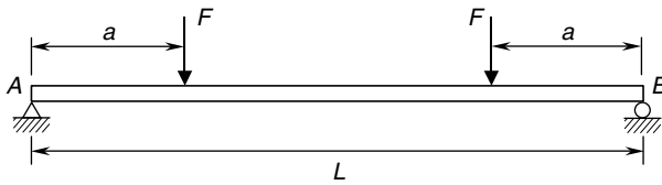
FIGURE 2.46 Twin concentrated forces.
