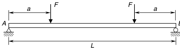
FIGURE 2.44 Twin concentrated forces.
