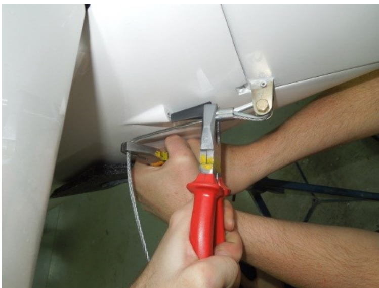
Fig. 27-6 Straighten of Steel Cable
