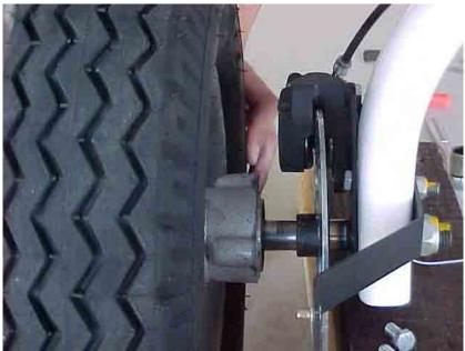
Figure 7.20 Wheel and spacer in assembly
