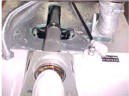
Once it is through the lower housing there should be a plastic washer then the metal washer and then the metal spacer tube.
