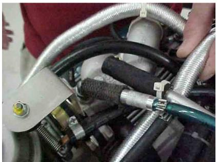
Figure 7.53 Insert left carb balance hose to left carb intake manifold
