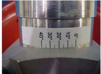
7. Adjust all blades to the same propeller pitch angle of attack.
