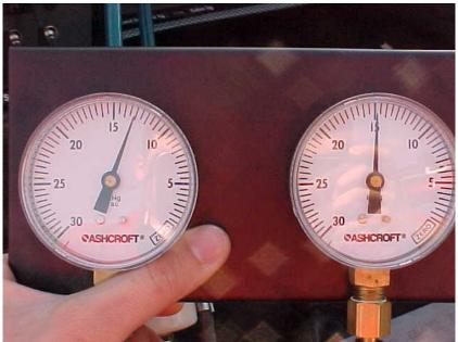
Figure 7.58 Initail reading of imbalanced manifold pressures
