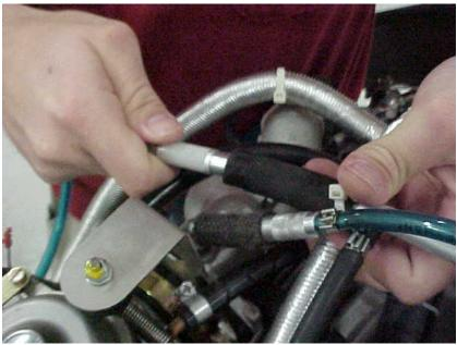
Figure 7.54 Insert right carb balance hose to end of compensation tube
