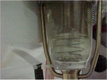
Figure 7.62: Fuel Filter Debris
