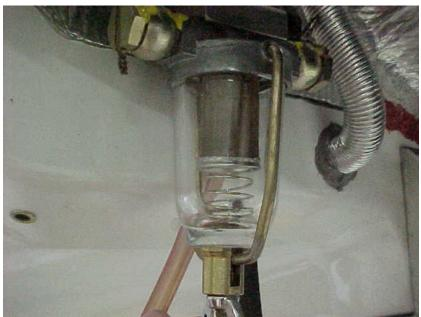
Figure 7.68: Fuel Filter supported by Spring
