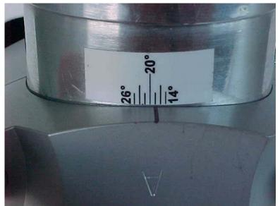
Figure 6.5 Pitch adjustment angles, later models, note: blade A at 18 deg.
