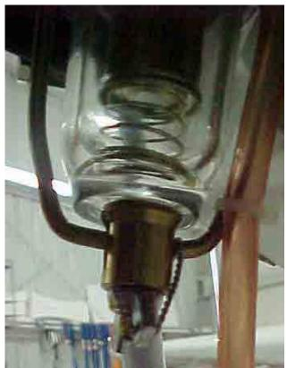
Figure 7.65: Fuel Filter Safety Wire
