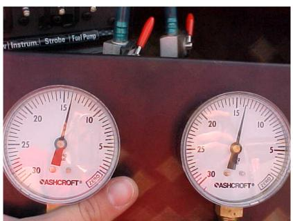
Figure 7.61 Balanced carb readings after adjustment
