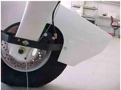
Figure 7.11 Main wheel with brake caliper
