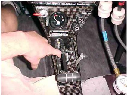
Figure 7.59 From the cockpit, access the throttle cables
