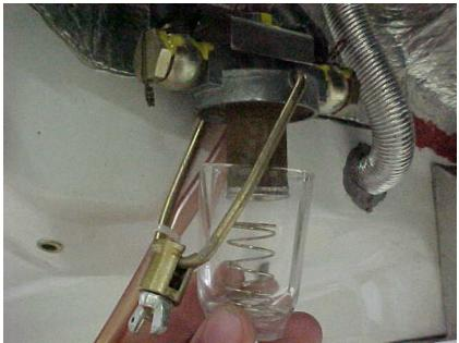
Figure 7.66: Fuel Filter Removed
