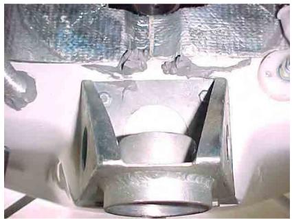
Figure 7.39 Lower nose strut bearing housing
