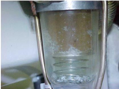
Figure 7.64: Fuel Filter Debris
