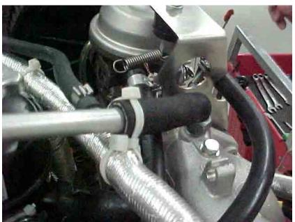
Figure 7.50 Carb support spring and clamp removed
