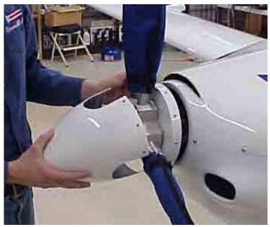
Figure 6.2 Removal of the spinner
