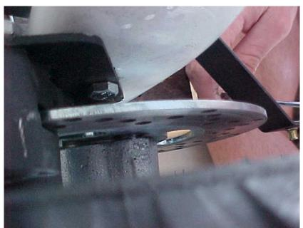
Figure 7.21 Tight tolerance of brake disk to wheel assembly
