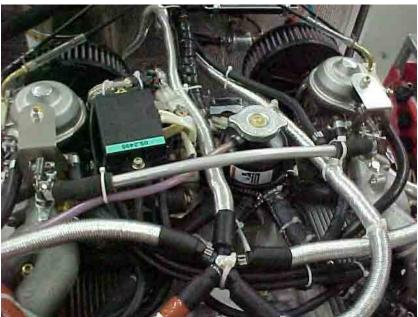
Figure 7.47 Crossover compensation tube between carbs
