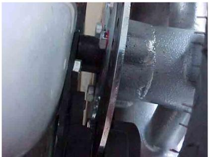
Figure 7.22 Brake disk mounted to wheel assembly
