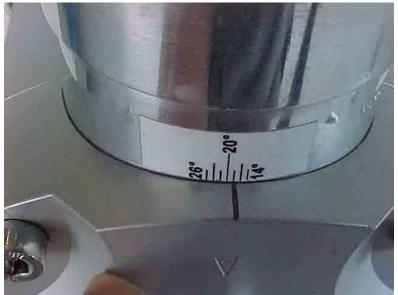
Figure 6.8 Checking blades A and B are also at 18 degrees
