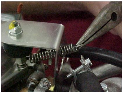
Figure 7.49 Carb support spring removed
