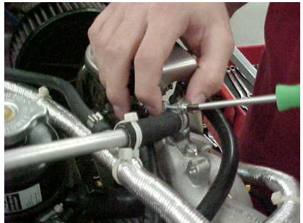
Figure 7.51 Removal of the hose clamp on the compensation tube.
