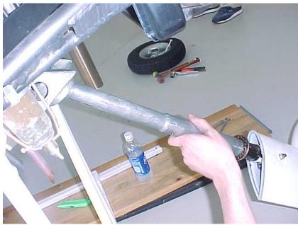
Figure 7.35 Nose strut being removed from firewall mounted bearing housings.
