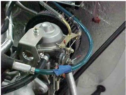
Figure 7.55 Balance hose inserted through compensation tube. Note tape ID of right hose to right carb
