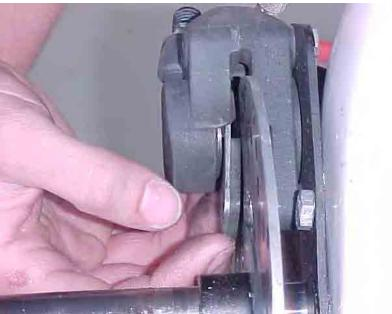
Figure 7.5 Brake pad removal
