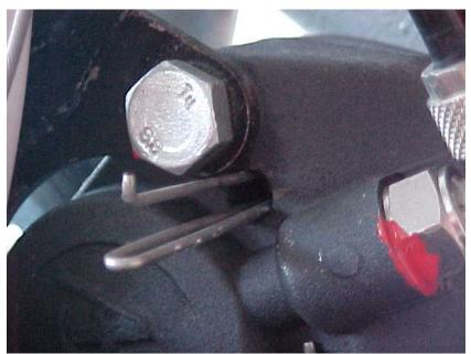
Figure 7.3 Brake pad retaining pin removed
