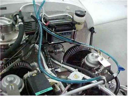
Figure 7.56 Secure hoses for engine test run
