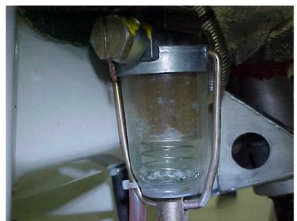
Figure 7.63: Fuel Filter Debris
