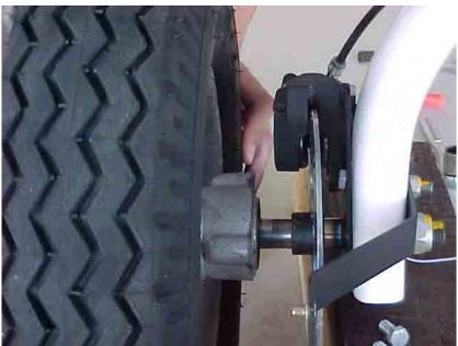
Figure 7.18 Main wheel sliding off the axle.
