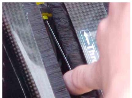
Figure 7.60 Detail of throttle cable access to change carb setting values
