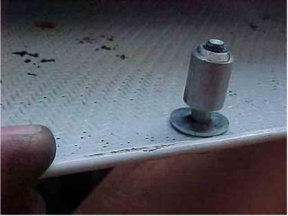
Figure 7.24 Main wheel pant outboard spacer to axle nut
