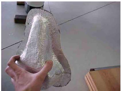
Figure 7.31 Nose strut firewall cover removed.
