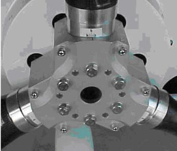
Figure 6.3 Six M4 and Six M8 bolts in hub
