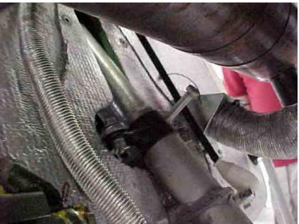
Figure 7.33 Nose strut bellcrank bolt removed
