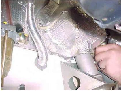
Figure 7.43 Reseal fire resistant material around the firewall cover.
