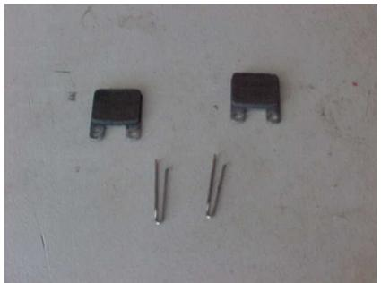
Figure 7.6 Brake pads and retaining pins
