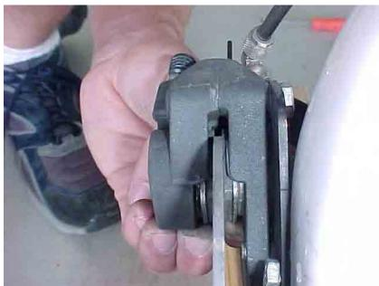
Figure 7.8 Brake pad repacement
