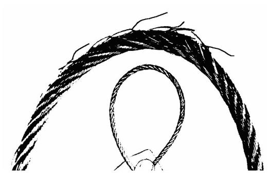
Figure 7.77 Wire cable strands exposed by bending the cable.
