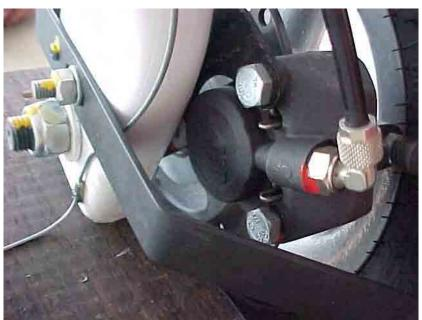
Figure 7.9 Brake pad retaining pins installed
