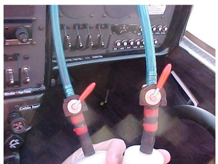
Figure 7.57 Balance shut offs are used to reduce needle fluctuations
