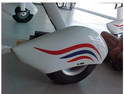
Figure 7.25 Main wheel pant installed Lift the wing again, remove blocks under the gear leg and lower the completed wheel assembly.
