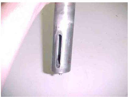
Figure 7.40 Nose strut upper tube showing movement slot
