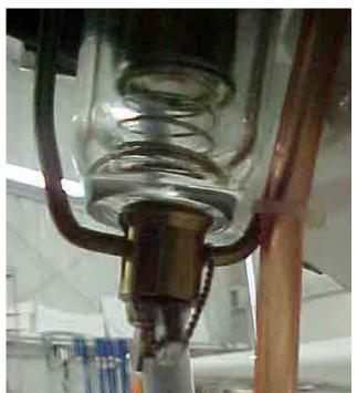
Figure 7.68: Fuel Filter Safety Wire Finally safety wire the wing nut.
