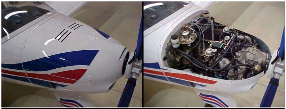
Figure 6.1 Cowling removal
