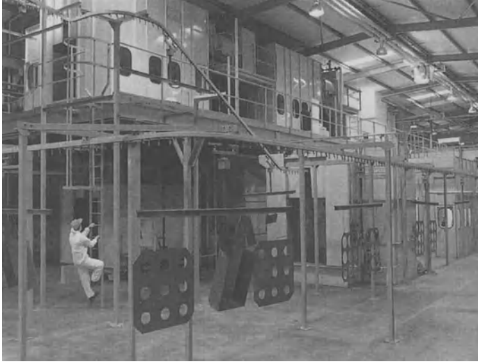
Fig. 2.21. Automated transportation of parts to either one of two painting systems, one for cast components and the other for sheet metalwork. [Courtesy of Yamazaki Mazak Ltd.]
