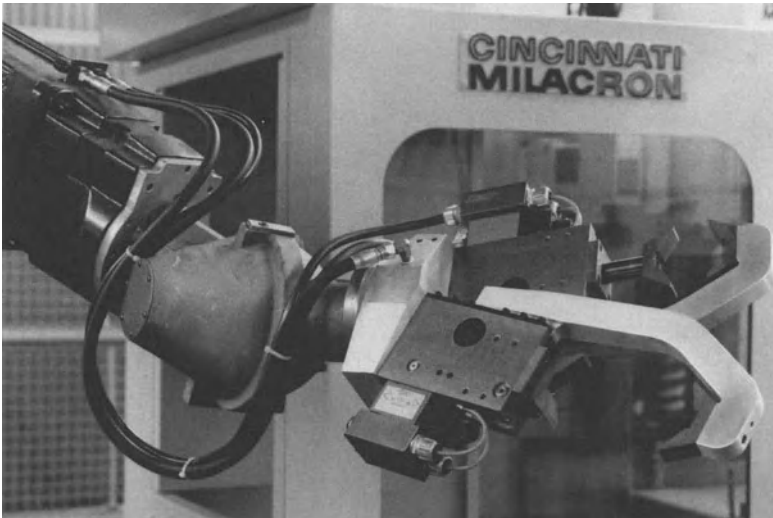
Fig. 2.7. Detail of the robot’s gripper in the “Southampton cell” designed by the author. The hydraulically operated and offset back-to-back gripper has synchronised movable jaws, enabling fast load/unload of the parts (i.e. of varying diameters) and close access to the workholding equipment. NB: Jaw faces/ends can be quickly changed. [Courtesy of Southampton Institute/Cincinnati Milacron.]
