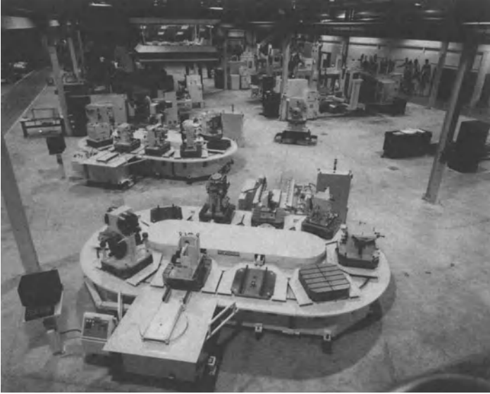
Fig. 2.8. An FMS illustrating "pallet pools" strategically positioned for easy access of the wire-guided AGVs. Note the elevated control room. [Courtesy of Cincinnati Milacron.]
