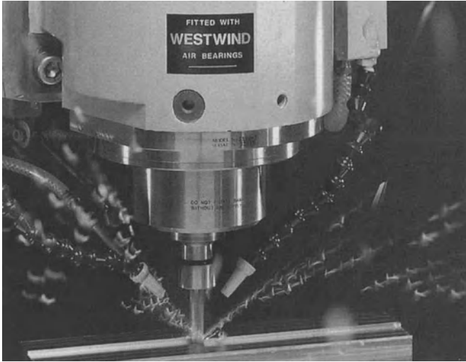
Fig. 2.25. Details of air-driven high-speed spindles used in milling applications. a A typical aerodynamic thrust bearing with spiral grooves. Air is dragged into the grooves by virtue of the relative motion of the plates and a pressure rise is caused by the restriction of the sealing band with consequent load generation. b A cutaway diagram of an air-driven spindle. c An ultra-high speed milling operation on an aluminium component. [Courtesy of Westwind Air Bearings Ltd.]
