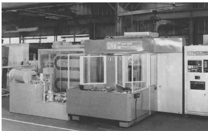
Fig. 1.51. A large 4-pallet machining centre (horizontal) with 4-axis control. [Courtesy of FMT Ltd.]
