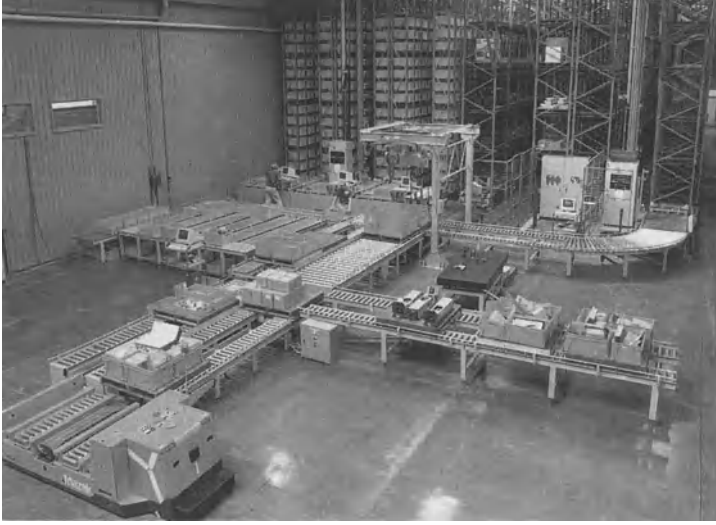
Fig. 2.18. The automatic warehouse under the “host’s” control, with two AGVs to distribute parts to assembly areas. [Courtesy of Yamazaki Mazak Ltd.]
