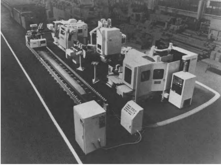
Fig. 2.5. Turning and vertical/horizontal machining centres in an FMC configuration together with robot-loading rail-guided vehicle. [Courtesy of Cincinnati Milacron.]
