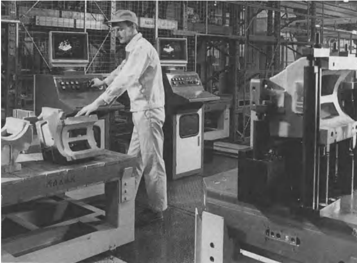
Fig. 2.15. Fixtures are scheduled by the host computer and all of its assembly details are displayed on the screen, allowing the assembler to speedily and accurately build up the part on its fixture. [Courtesy of Yamazaki Mazak Ltd.]
