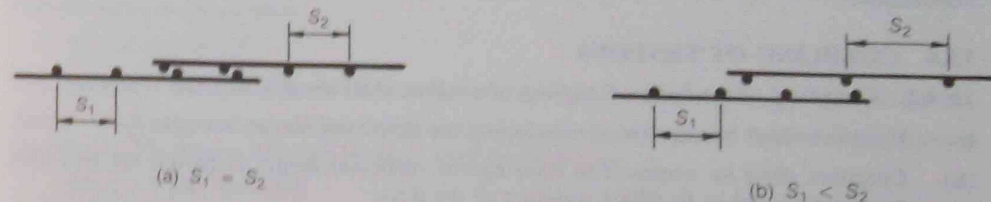
FIGURE 13.2.4 LAPPED SPLICES FOR FABRIC
