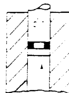
Fig 4 Bridgman 'unsupported area' plug seal.
