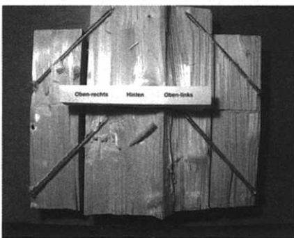
Figure 17.21 Lap joint with self-tapping screws. Left: inclined screw arrangement; right: screws perpendicular to the member surface
