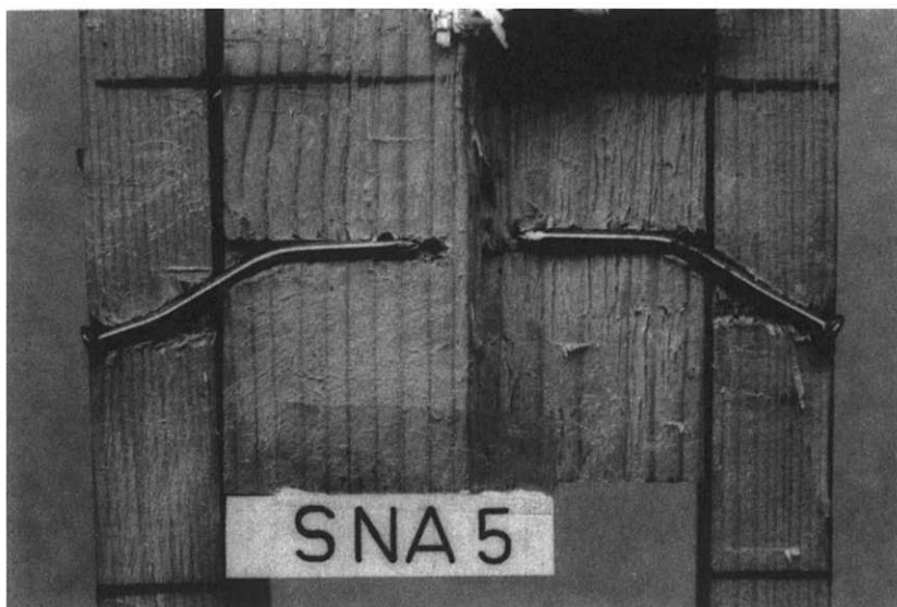
Figure 17.1 Opened nailed connection after a test to determine the load-carrying capacity
