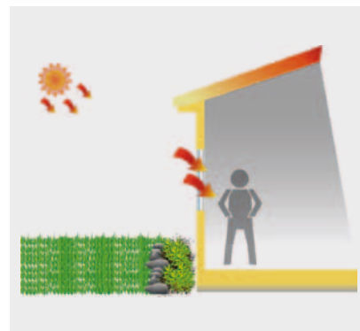
Solar Heat Gain Co-efficient [ SHGC_w ] is a measure of solar radiation entering through the window system.
