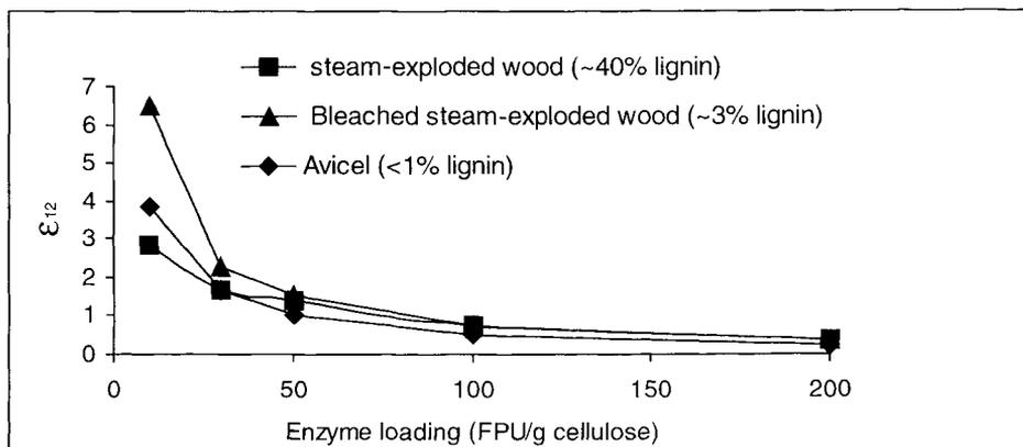
Figure 4. Conversion efficiency at the 12<sup>th</sup> h ( $\epsilon_{12}$ ) of enzymatic hydrolysis of Avicel and steam-exploded Douglas fir wood, with and without bleaching, under various enzyme loadings.  $\epsilon_{12} = \{\text{conversion yield @ 12 h}\} / \{\text{FPU enzyme added}\}$ .
