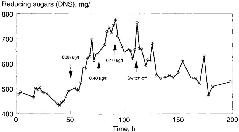
Figure 2. Concentration of soluble carbohydrates in white water samples taken from the bow screen during the first mill trial.
