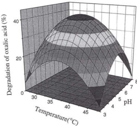
Figure 2. Response surface showing the effect of temperature and pH on the degradation of oxalic acid by oxalate decarboxylase. The figure shows a 30 min reaction with 990 mU oxalate decarboxylase per  $\mu$ mole oxalic acid.  $R^2=0.86$ ,  $Q^2=0.45$ , RSD (residual standard deviation)=7.3.
