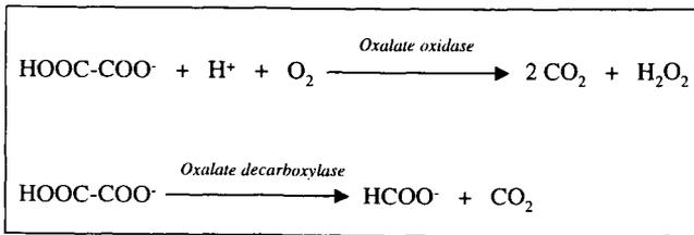
Figure 1. Reactions catalysed by oxalate oxidase and oxalate decarboxylase.
