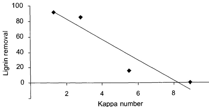
Figure 3. Correlation between kappa number and Py-GC-MS estimation of lignin removal from flax pulp after  $LMS_{HBT}$  treatment followed by E and EP stages.
