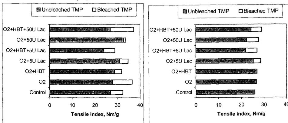
Figure 1. Evolution of tensile index after different treatments with laccases applied on primary-refined (left) or secondary-refined (right) softwood TMP at 90 ml CSF.
