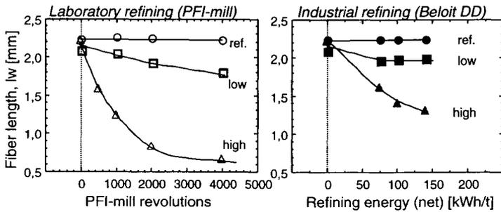
Figure 4. Fiber length of enzyme-treated pulps vs. energy input in PFI-mill refining (left diagram) and industrial refining (right diagram).
