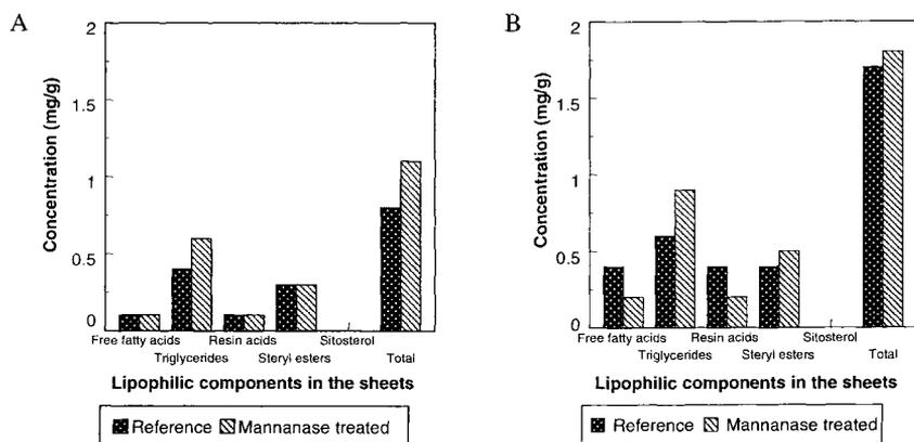
Figure 2. Analysis of the extractives content in the sheets after mannanase treatment of DCS fraction (A) or 1 % TMP pulp suspension (B). Enzyme dosages: 10 nkat/ml DCS fraction, 1000 nkat/g pulp. Treatment conditions: 2 h, pH 5, 50°C.
