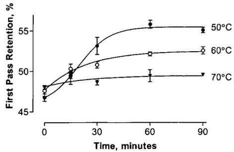
Figure 2. Effect of temperature on Iogen BRC kinetics. Headbox stock was treated with 100 cellulase U/L. FPR was measured with addition of Bufloc 594 at 0.5 kg/t, a 45 mesh screen, and stirring at 1000 rpm. Data are means of 3 replicates ± standard errors.
