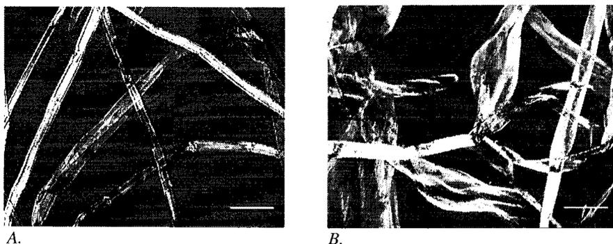
Figures 3A-B. Stirring of WU1 after 1h under non-shearing (A, non-affected fibres with dislocations) and shearing conditions (B, many partly disintegrated fibres without dislocations). Polarised light microscopy. Scale bars 50  $\mu\text{m}$ .
