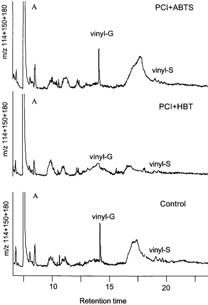
Figure 2. Py-GC-MS chromatograms of pulps treated with *Pycnoporus cinnabarinus* laccase in the presence of ABTS and HBT compared with the control. The sum of three single ions corresponding to the molecular ions of the cellulose marker (A, 4-hydroxy-5,6-dihydro(2H)-pyran-2-one, 114 m/z), and two main lignin markers, 4-vinylguaiacol ( $m/z$  150) and 4-vinylsyringol ( $m/z$  180), is represented.
