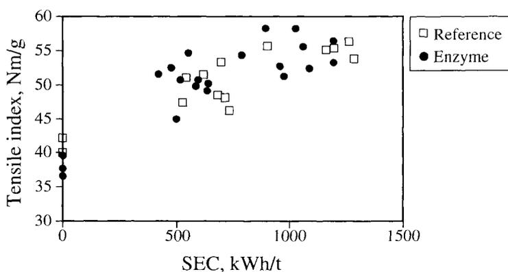
Figure 9. Tensile index of the handsheets as a function of SEC.
