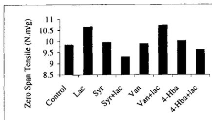
**Figure 7.** Zero Span Measurements of High-Kappa Pulpes Treated with Laccase and Phenolic Acids
