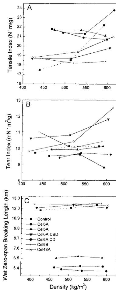
**Figure 2.** Properties of handsheets prepared from cellulase-treated kraft pulps without refining
