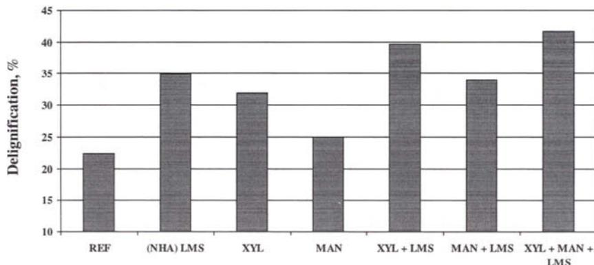
Figure 3. Simultaneous treatments of kraft pulp with xylanase, mannanase and LMS, using NHA as mediator; delignification after alkaline extraction of lignin. Original kappa number 23.5.
