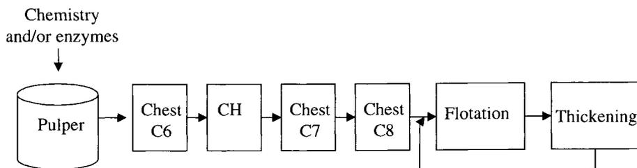
Figure 1. The pilot deinking loop used in the experiments. After pulping the pulp was sent to the retention chest C6. The pulp was screened (Lamort CH screen, 20/100 slots) before transfer to the chest C8 prior to flotation and thickening.
