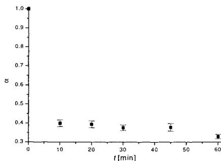
Figure 3. Development of quenching factor  $\alpha$  with  $t$  for the laccase-ABTS system.
