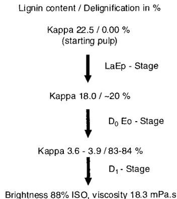
**Figure 7.** Flowsheet of delignification and viscosity changes during laccase/mediator ECF bleaching.
