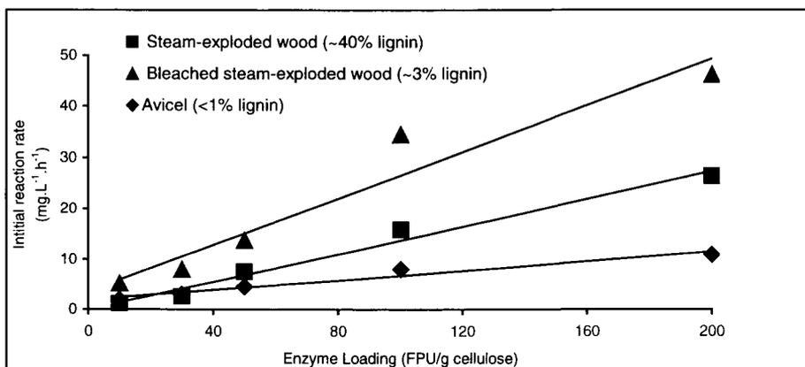
Figure 3. The initial reaction rates during the enzymatic hydrolysis of Avicel and steam-exploded Douglas fir wood (with and without bleaching) under various enzyme loading.
