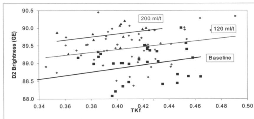
Figure 10. Northern softwood with O<sub>2</sub> delignification (1000 ton/day). After an initial gain in brightness was achieved with 120 ml/t of xylanase, the dosage was increased to 200 ml/t and a bigger benefit was observed.
