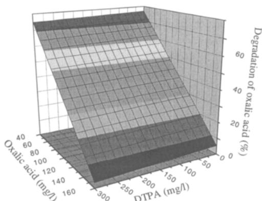
Figure 5. Response surface showing the effect of dilution and DTPA addition on the degradation of oxalic acid in a Z-stage filtrate by oxalate oxidase.
