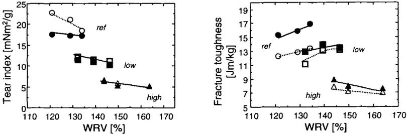
Figure 11. Tear index (geom. mean) and fracture toughness index (geom. mean) as a function of WRV for machine-made sheets (open symbols) and handsheets (filled symbols).
