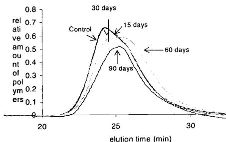
Figure 4. HPSEC of alpha-cellulose tricarbanilates prepared from *P. taeda* biotreated by *C. subvermispora*
