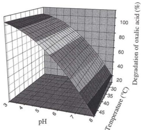
Figure 3. Response surface for the degradation of oxalic acid by oxalate oxidase. The figure shows a reaction with 347 mU oxalate oxidase per  $\mu$ mole oxalic acid.  $R^2=0.99$ ,  $Q^2=0.89$ , RSD=5.7.
