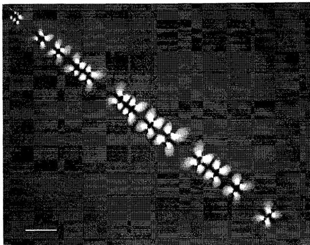
Figure 8. Balloons as "string of pearls" in pulp fibre WU6 swollen in phosphoric acid. Scale bar 50  $\mu\text{m}$ .
