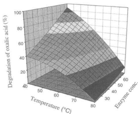
Figure 4. Model of a 15 min degradation of oxalic acid by oxalate oxidase showing the effect of temperature and enzyme concentration (mU/ $\mu$ mole).
