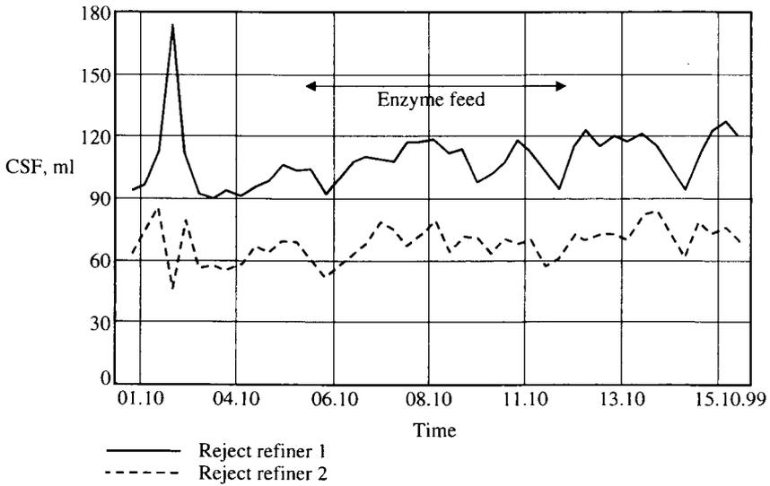
Figure 5. Freeness (CSF) of the pulp after the reject refiners during the second trial..
