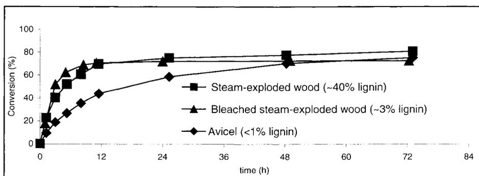
Figure 2. Enzymatic hydrolysis of Avicel and steam-exploded Douglas fir wood (with and without bleaching) at 50 FPU/g cellulose enzyme loading.
