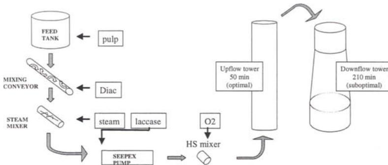
**Figure 4.** Optimized addition points for laccase and mediator in pilot plant.
