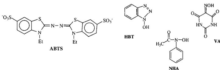
Figure 1. Commonly employed mediators for LMS biobleaching of kraft pulps.
