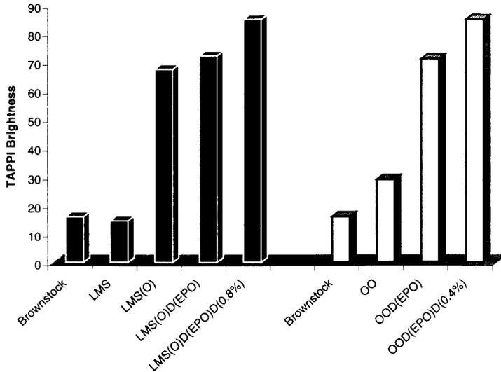
Figure 9. Brightness development for bleaching kappa 27.5 SW kraft pulp via  $LMS_{VA}OD(E+P+O)D$  and  $OOD(E+P+O)D$ .
