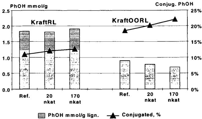
Figure 2. The effect of laccase on the content of phenolic hydroxyl groups. Lignin concentration 0.15mg/ml, laccase charge 20 and 170 nkat/mg.
