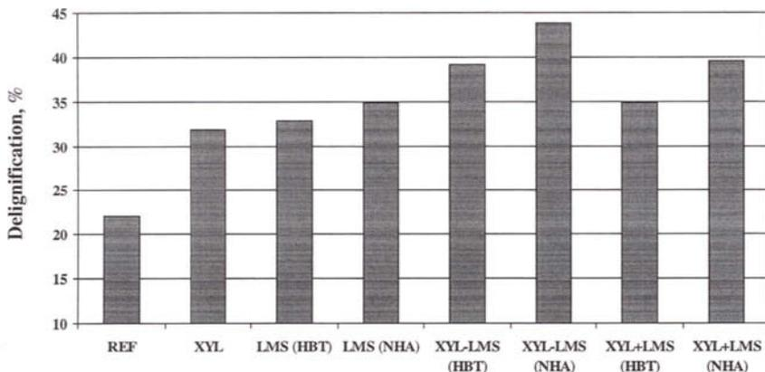
Figure 2. Sequential and simultaneous treatments of kraft pulp with xylanase and LMS, delignification after alkaline extraction of lignin. Original kappa number 23.5.
