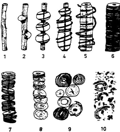
Figure 6. Different steps (1-10) in swelling, ballooning, spiral band formation and disintegration of a carboxymethylated cellulose fibre (Stawitz and Kage 1959; Jayme and Harders-Steinhäuser 1964).
