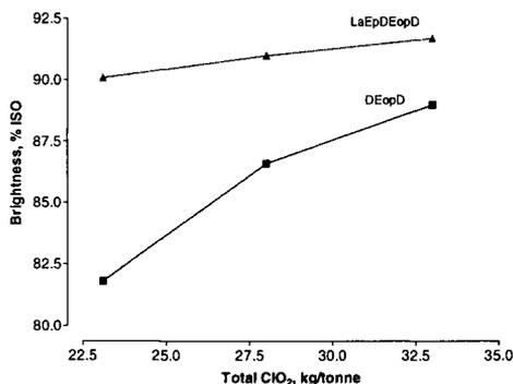
Figure 2. Laboratory-scale bleaching of kraft pulp by laccase and NHA (0.5% on pulp).
