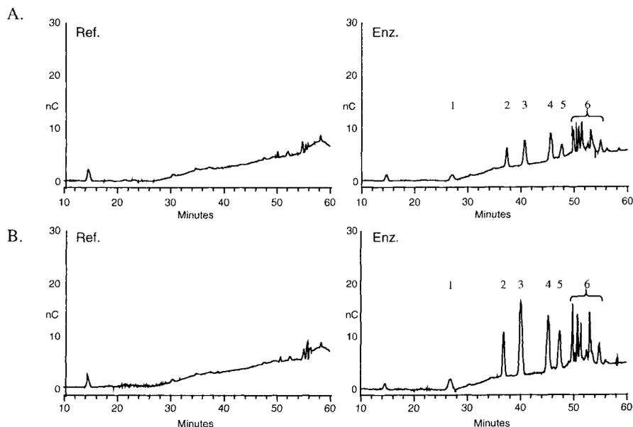
Figure. 1. HPLC analysis of the oligosaccharides liberated in the mannanase treatment of DCS fraction (A) and 1% TMP pulp suspension (B). Enzyme dosages: 10 nkat/ml DCS fraction, 1000 nkat/g pulp. Treatment conditions: 2 h, pH 5, 50°C. Peak identification: 1, Man; 2, Man<sub>2</sub>; 3, Man<sub>3</sub>; 4, Man<sub>4</sub>; 5, GalMan; 6, Man<sub>5</sub>, Gal<sub>2</sub>Man<sub>5</sub>, Man<sub>6</sub>, GalMan<sub>3</sub> (19).
