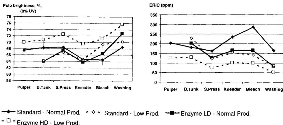
Figure 3. Development of brightness (a) and residual ink content (b) of the pulps during the deinking process. LD low dosage, HD high dosage.
