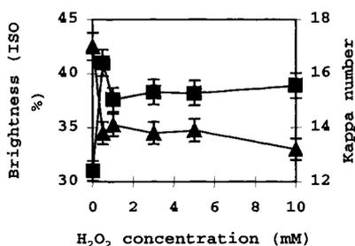
Fig. 6 Effect of hydrogen peroxide concentration on bleaching of UKP the crude enzyme solution containing 20 U MnP of MG-60 at 37°C for 24 h. (brightness (■) and kappa number (▲))
