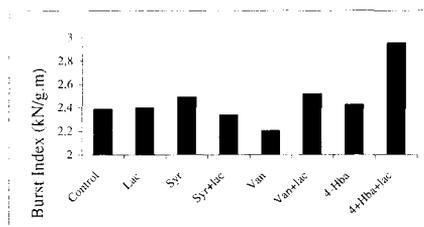
**Figure 3:** Burst Index Measurements of High-Kappa Pulps Treated with Laccase and Phenolic Acids
