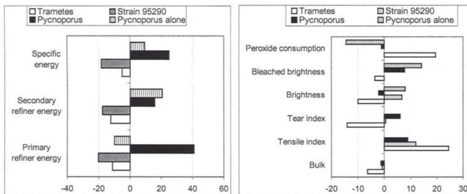
Figure 8. Effect of laccase-mediator treatment of wood chips on energy consumption and TMP quality.
