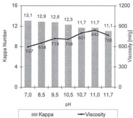
Figure 3. pH dependence of kappa numbers and viscosities after the bleaching sequence Cu-E.
