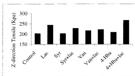
**Figure 5.** Z-direction Tensile Measurements of High-Kappa Pulps Treated with Laccase and Phenolic Acids
