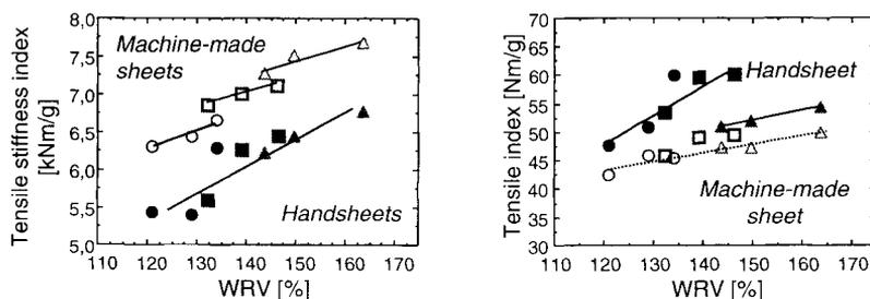
Figure 10. Tensile stiffness index and tensile index for the industrially refined pulps as a function of WRV. Machine-made sheets has open symbols and geometric means for MD and CD strength are used. Handsheets have filled symbols. Legend: reference●, low enzyme charge■ and high enzyme charge▲.
