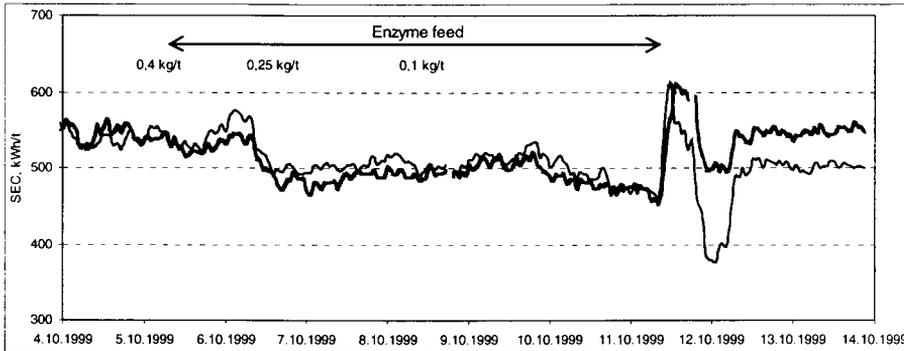
Figure 7. The specific energy consumption (SEC) of the reject refiners during the second trial.
