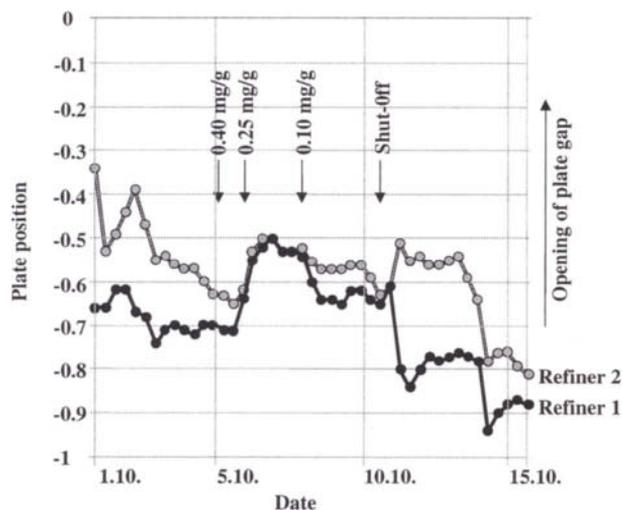
Figure 6. Plate position of the refiners during the second trial. Changes in the dosage of the enzyme are shown in the figure.
