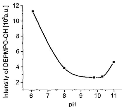
Figure 5. pH course of the relative intensity of the OH-radical spin adduct obtained with copper/ 4-AP/ H<sub>2</sub>O<sub>2</sub>.
