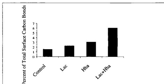
Figure 1. ESCA Analysis of Handsheets from High-Yield Kraft Pulp Fibers Treated with Laccase and 4-Hydroxybenzoic Acid (4-Hba) to Determine Surface Acid Group Content (ESCA analysis performed after 12 hours of Soxhlet extraction with acetone) [15]
