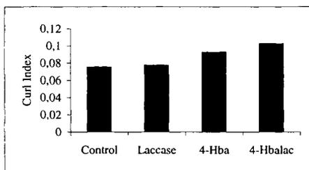
**Figure 6.** Curl Index Measurement of High-Kappa Pulpes Treated with Laccase and 4-Hydroxybenzoic Acid Performed on a Fiber Quality Analyzer
