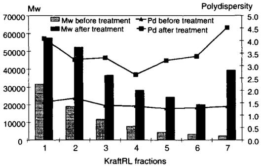
Figure 9. Changes in weight average molar mass and polydispersity of KraftRL fractions in the laccase treatments. Lignin concentration 0.13 mg/ml, laccase charge 170 nkat/mg.
