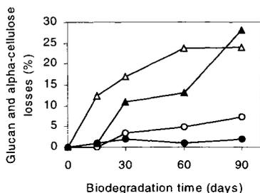
Figure 3. Glucan (-●-) and alpha-cellulose (-▲-) losses during biopulping of *P. taeda* (filled symbols) and *E. grandis* (open symbols) by *C. subvermispora* (24).
