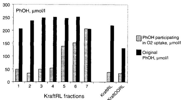
Figure 10. Comparison between the original, determined PhOH-group content and the theoretically oxidized content calculated from the oxygen consumption.
