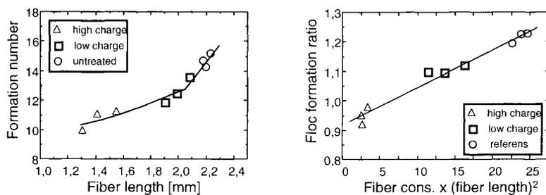
Figure 9. Formation number decreased with decreasing fiber length. Floc formation ratio was linearly related to fiber consistency  $\times$  (fiber length)<sup>2</sup> as predicted by Kerekes crowding number.
