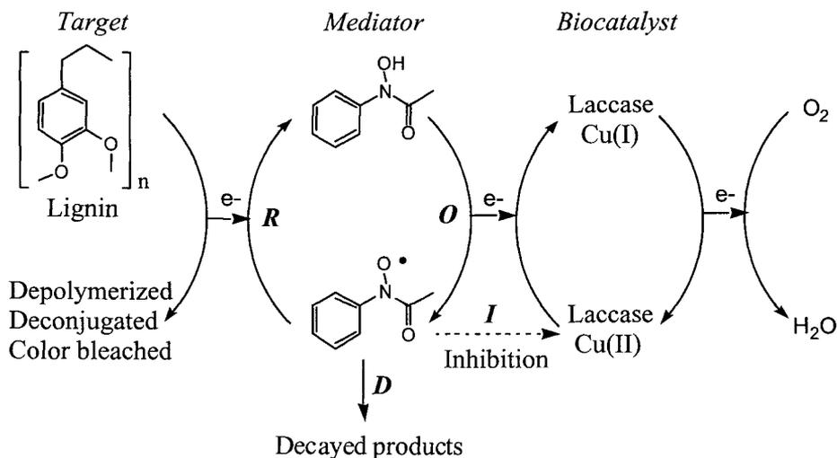
Figure 2. Generalized mechanism for mediated biocatalysis of laccase. During the catalysis, the mediator is first oxidized by laccase (reaction *O*), then the oxidized mediator is reduced by target molecule (reaction *R*) to be regenerated for next round mediation. The oxidized mediator may decay into inactive byproducts (reaction *D*) or inactivate laccase (reaction *I*), diminishing the overall mediation/catalysis efficiency.
