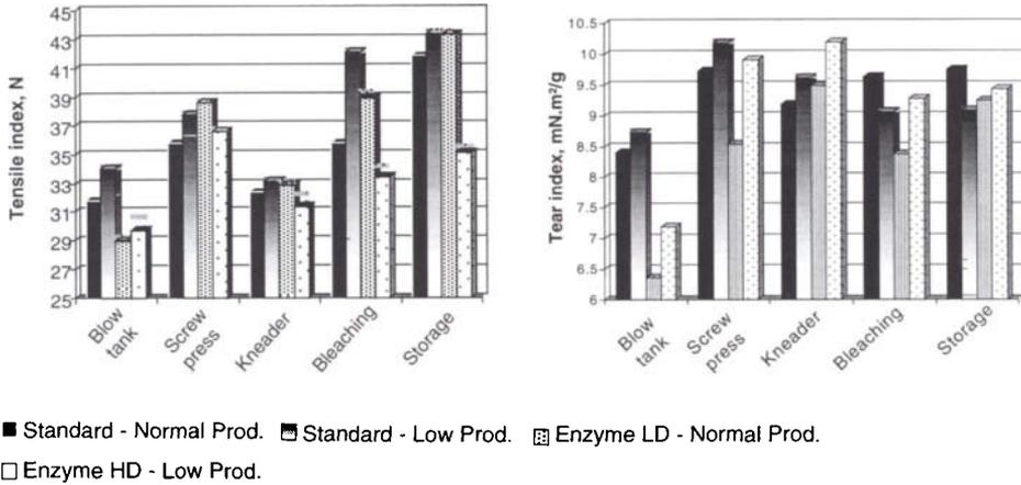
Figure 4 . Development of tensile index (a) and tear index (b) of the pulps during the deinking process.
