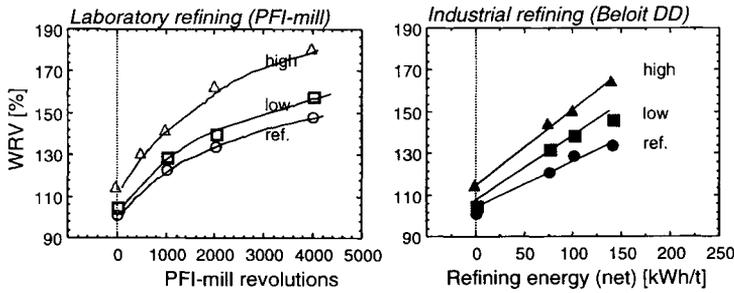
Figure 3. WRV of enzyme-treated pulps vs. energy input in PFI-mill refining (left diagram) and industrial refining (right diagram).
