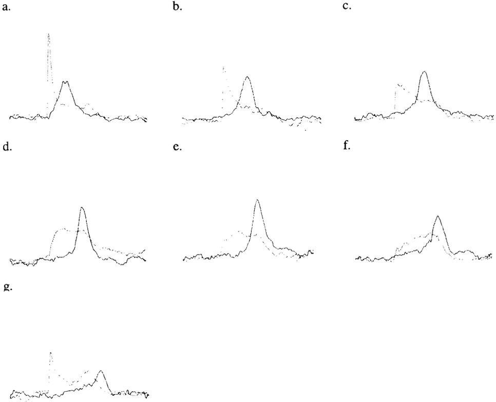
Figure 8. GPC elution curves of the KraftRL fractions before ----- and after - - -laccase treatment. Lignin concentration 0.13 mg/ml, laccase charge 170 nkat/mg. Fr1 (a); fr2 (b); fr3 (c); fr4 (d); fr5 (e); fr6 (f) and fr7 (g).
