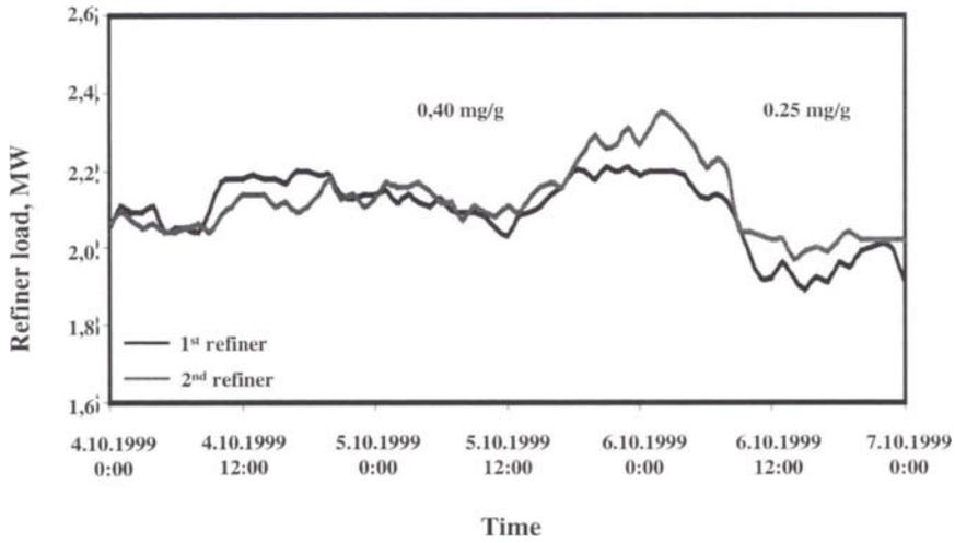
Figure 4. Data on motor loads of the refiners at the beginning of the second trial.
