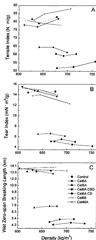
**Figure 4.** Properties of handsheets prepared from cellulase-treated kraft pulps after 2000 revolutions PFI refining.
