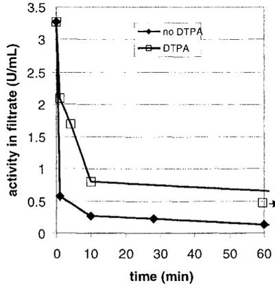
**Figure 3.** Loss of laccase activity at the high shear mixer. For the DTPA curve, a data point at 240 min was used to plot the graph. The high shear mixer was based on the design of GL&V, and was run at 3600 rpm.
