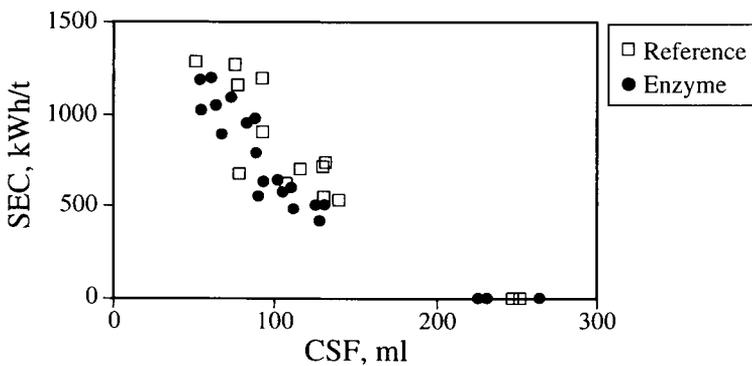
Figure 8. Energy consumption (SEC) and CSF during the enzyme and reference periods as obtained in the additional refining tests.
