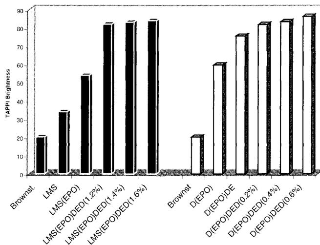
Figure 7. Brightness development for bleaching kappa 27.5 SW kraft pulp via LMS<sub>VA</sub>(E+P+O)DED and D(E+P+O)DED.
