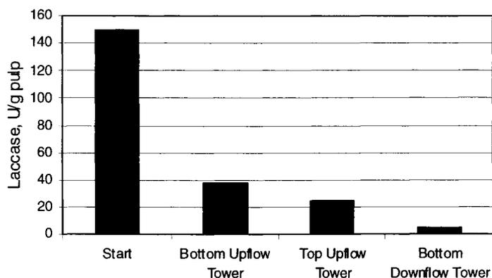
**Figure 5.** Residual laccase activity at various locations within pilot-plant after optimization of enzyme addition point.
