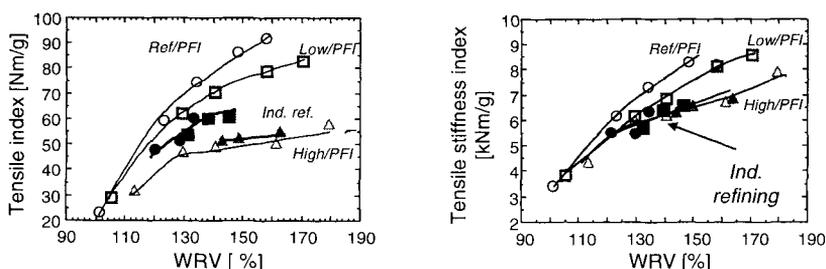
Figure 5. Tensile index and tensile stiffness index vs. water retention values for handsheets made from laboratory refined pulps (open symbols) (PFI) and industrially refined pulps (filled symbols). Legend: reference ●, low enzyme charge ■ and high enzyme charge ▲.
