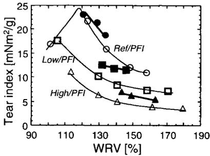
Figure 6. Tear index vs. WRV for handsheets made from laboratory and industrially refined pulps. Symbols see Fig 5.
