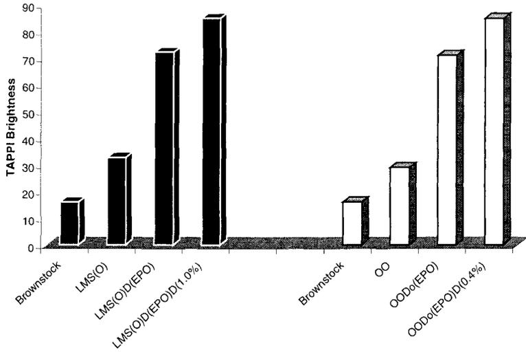
Figure 10. Brightness development for bleaching kappa 50.0 SW kraft pulp via  $LMS_{VA}OD(E+P+O)D$  and  $OOD(E+P+O)D$ .
