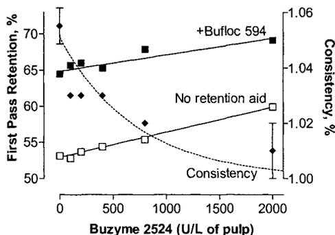
Figure 3. Effect of xylanase Buzyme 2524 dose on consistency (◆) and retention (■,□). Mill A headbox stock was treated with enzyme for 1 h at 50°C. FPR was measured with a 70 mesh screen. Bufloc 594 was added at 2 kg/t when indicated.
