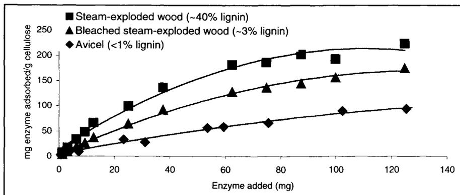
Figure 1. Adsorption of cellulase enzymes onto Avicel and steam-exploded Douglas fir wood (with and without bleaching).
