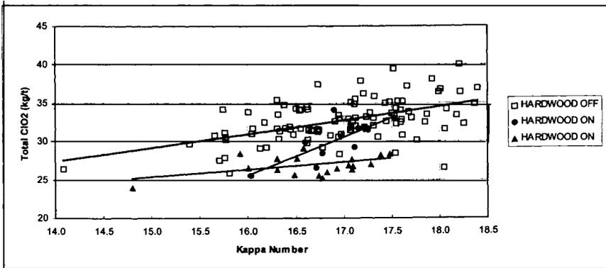
Figure 7. US hardwood mill: total ClO<sub>2</sub> versus Kappa number. In the initial stages of the enzyme trial, ClO<sub>2</sub> savings were moderate (circles). A higher level of savings was achieved after the Do set point was changed (triangles).
