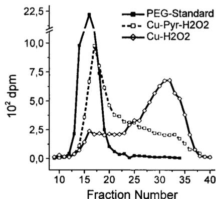
Figure 2. Depolymerisation of  $^{14}\text{C}$ -labeled polyethylene glycol by copper/  $\text{H}_2\text{O}_2$  in the presence and absence of pyridine.
