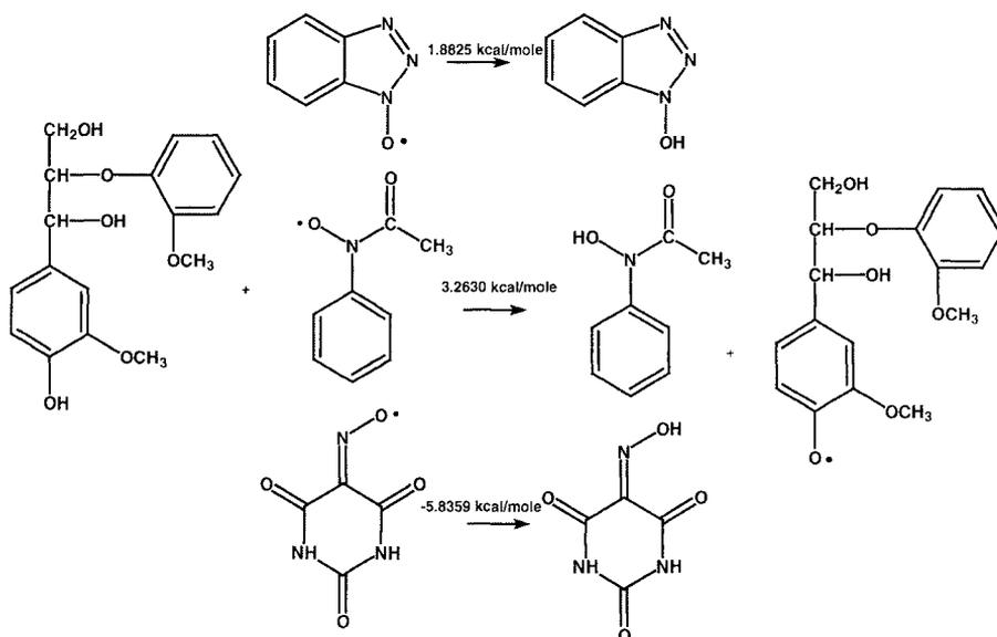
Figure 5. Computational results from modeling the oxidation of a model dilignol by the action of the  $RR'NO\bullet$  radical from VA, HBT, and NHA.
