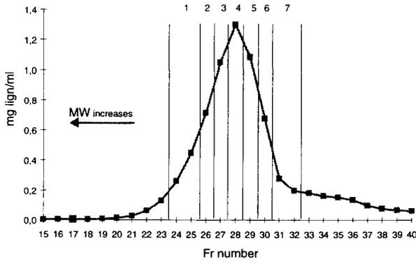
Figure 5. The fractionation of KraftRL and the fractions chosen for the experiments.
