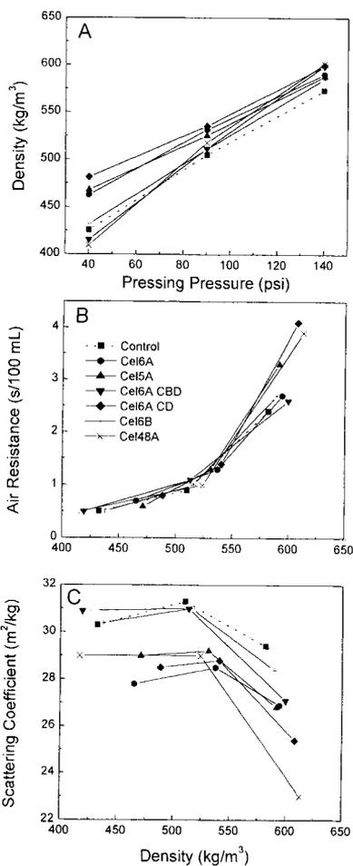
**Figure 1.** Properties of handsheets prepared from cellulase-treated kraft pulps without refining
