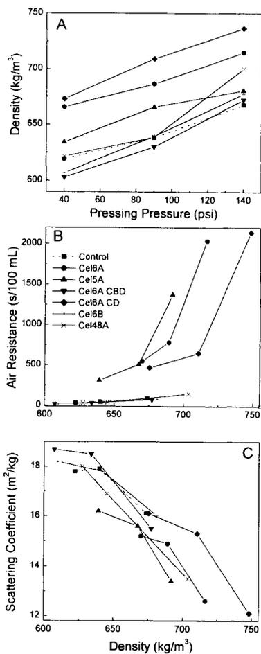
**Figure 3.** Properties of handsheets prepared from cellulase-treated kraft pulps after 2000 revolutions PFI refining.
