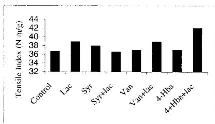
**Figure 4.** Tensile Index Measurements of High-Kappa Pulps Treated with Laccase and Phenolic Acids
