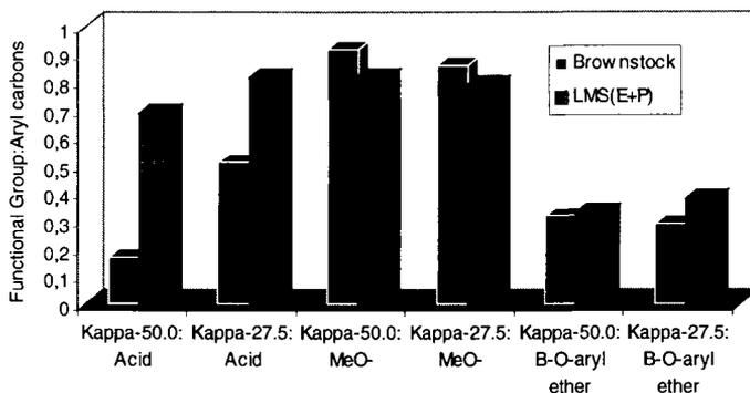
Figure 4. Changes in acid group, methoxyl, and  $\beta$ -O-aryl ether content of residual lignin isolated from kappa 50.0 and kappa 27.5 brownstocks and after  $LMS_{VA}(E+P)$  treatments, as determined by  $^{13}C$  NMR.
