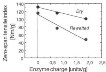
Figure 2. Zero-span tensile index for dry and rewetted sheets vs. enzyme charge.
