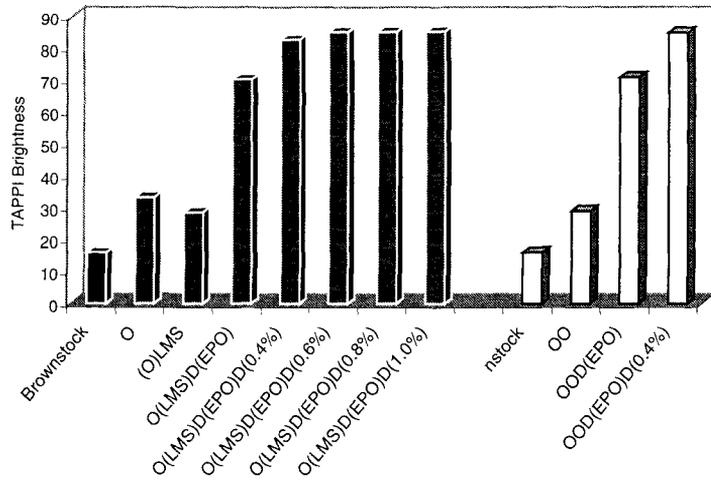
Figure 11. Brightness development for bleaching kappa 50.0 SW kraft pulp via  $O(LMS_{VA})D(E+P+O)D$  and  $OOD(E+P+O)D$ .
