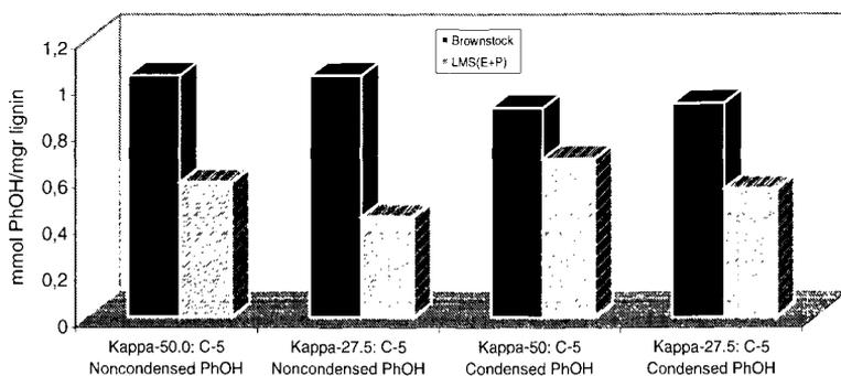
Figure 2. Changes in C-5 condensed and noncondensed phenolic guaiacyl content of residual lignin isolated from kappa 50.0 and kappa 27.5 brownstocks and after LMS<sub>VA</sub>(E+P) treatments, as determined by phosphorylation and <sup>31</sup>P NMR analysis.
