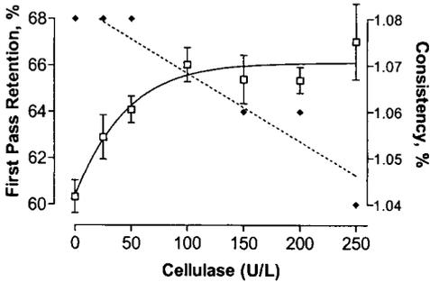
Figure 1. Effect of Iogen BRC dose on consistency(◆) and FPR(□). Headbox stock was treated with enzyme for 1 h at 50°C. FPR was measured with addition of Bufloc 594 at 0.5 kg/t, a 45 mesh screen, and stirring at 1000 rpm. Data are means of 3 replicates ± SE.
