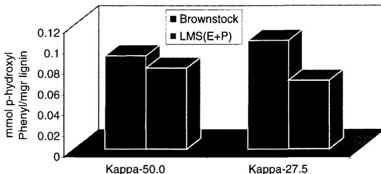
Figure 3. Changes in p-hydroxyl phenyl content of residual lignin isolated from kappa 50.0 and kappa 27.5 brownstocks and after  $LMS_{VA}(E+P)$  treatments, as determined by phosphorylation and  $^{31}P$  NMR.
