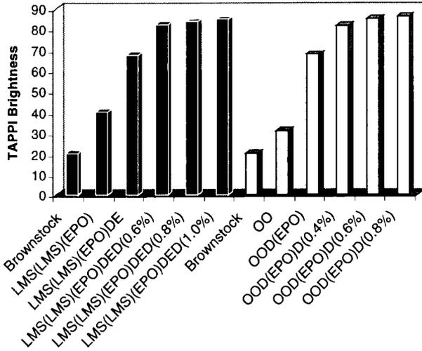
Figure 8. Brightness development for bleaching kappa 27.5 SW kraft pulp via  $LMS_{VA}LMS_{VA}(E+P+O)DED$  and  $OOD(E+P+O)D$ .
