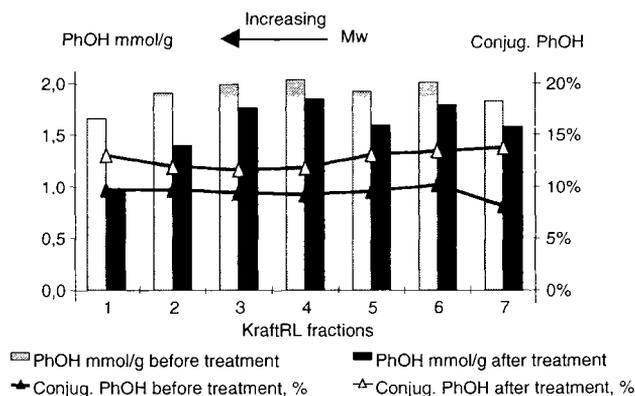
Figure 7. The effects of laccase on the content of phenolic hydroxyl groups. Lignin concentration 0.13 mg/ml, laccase charge 170 nkat/mg.
