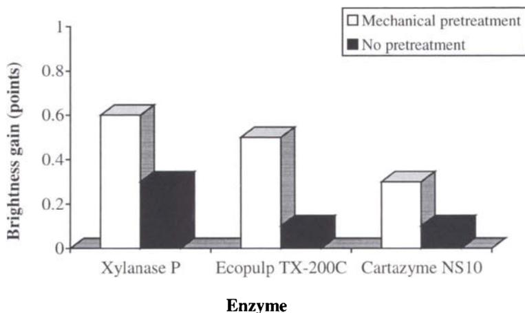
Figure 4. Impact of mechanical pretreatment on X-DED bleaching of bagasse pulp (1 U/g; kf of 0.75).
