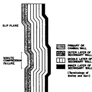
Figure 1. Slip plane and minute compression failure (Wardrop and Dadswell 1947; Keith and Côté 1968).
