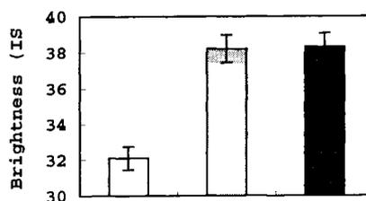
Fig. 7 Comparison of brightness increase after 3 hours enzyme bleaching with continuous (■) or initial (▨) addition of hydrogen peroxide. (control: □)
