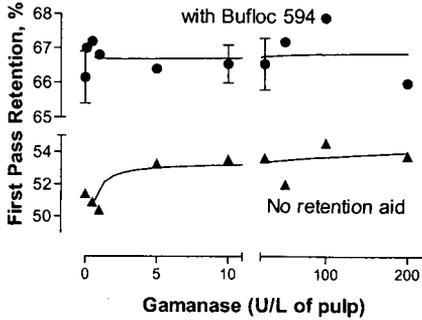
Figure 5. Effect of mannanase dose on retention of newsprint stock. Headbox stock was treated with enzyme for 1 h at 50°C. FPR was measured with Bufloc 594 at 0 or 2 kg/t, and a 70 mesh screen. Data are means of 1-3 replicates ± standard errors.
