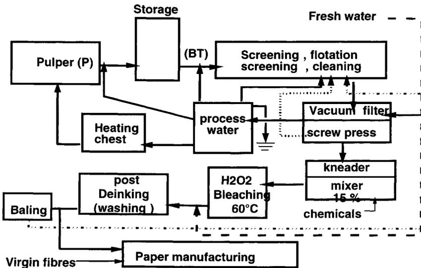
Figure 2. Deinking line of Moulin Vieux mill. BT, blow tank.
