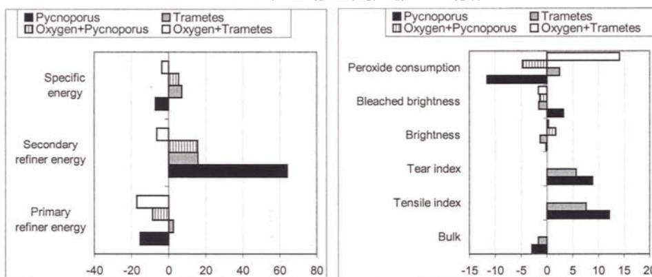
Figure 9. Effect of laccase treatment of wood chips on energy consumption and TMP quality under oxygen pressure or omitting oxygen pressure.
