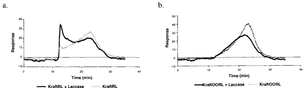
Figure 3. GPC elution curves of KraftRL (a) and KraftOORL (b) before and after laccase treatment. Lignin concentration 1.5 mg/ml, laccase charge 20 nkat/mg.
