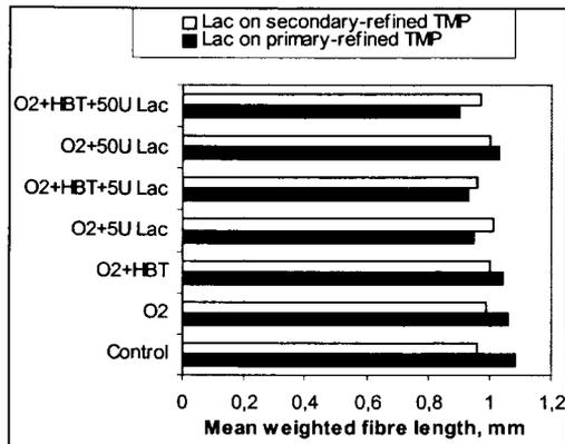
Figure 3. Evolution of mean length of fibres after different treatments with laccases applied on primary-refined or secondary-refined softwood TMP at 90 ml CSF.
