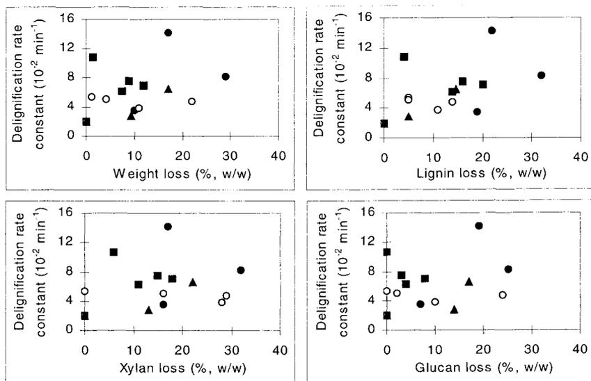
Figure 1. Delignification rate constants for the bulk phase as a function of wood weight and component losses caused by the fungal pretreatment. Fungal pretreatments with *Trametes versicolor* (●), *Punctularia artropurpuracens* (■), *Phanerochaete chrysosporium* (▲) and *Wolfiporia cocos* (○) (reproduced from ref. 7).
