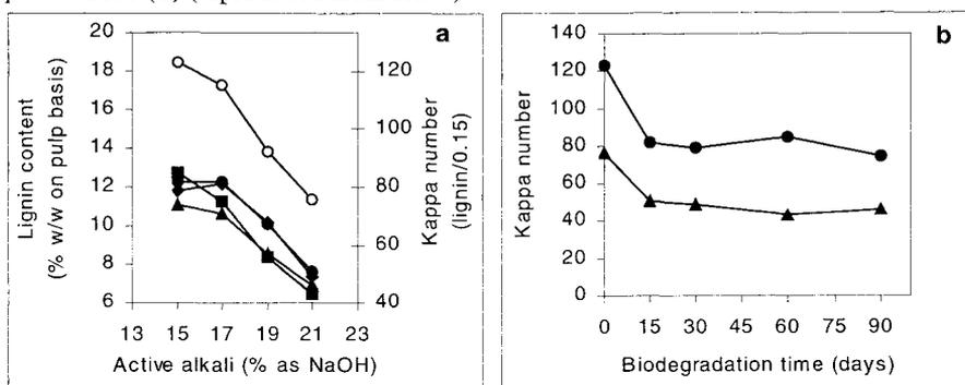
Figure 2. (a) Residual lignin contents in high-yield kraft pulps from *P. taeda*. Undecayed control (○) and samples biotreated by *C. subvermisporea* for 15 (●), 30 (◆), 60 (◻) and 90 (▲) days. (b) Pulps from a 15-day biotreated sample cooked with 15% (●) and 21% (▲) of active alkali. In both cases, 25% sulfidity and a 35-minute cooking at 170°C.
