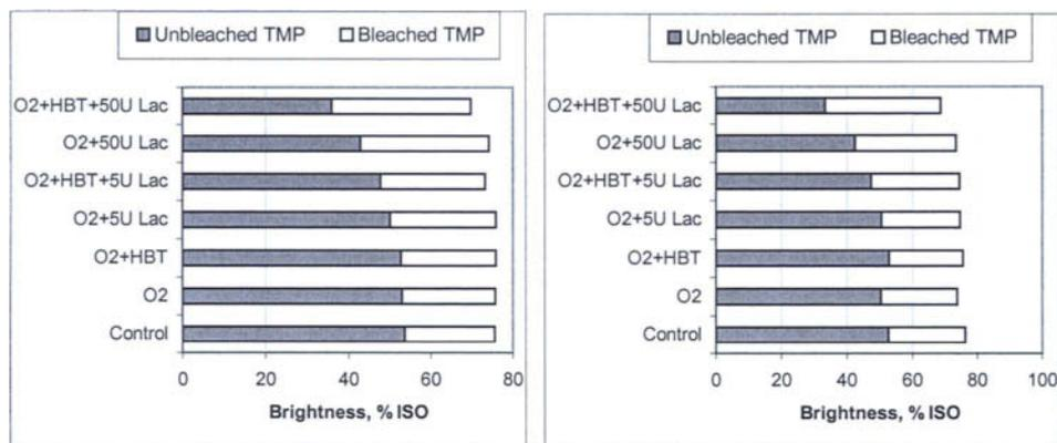
Figure 4. Evolution of brightness after different treatments with laccases applied on primary-refined (left) or secondary-refined (right) softwood TMP at 90 ml CSF.
