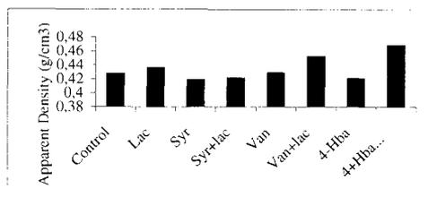
**Figure 2:** Apparent Density Measurements of High-Kappa Pulps Treated with Laccase and Phenolic Acids
