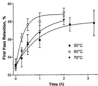
Figure 4. Temperature effects on kinetics of retention improvement by Buzyme 2524. Mill A headbox stock was treated with 1000 xylanase U/L. FPR was measured with no retention aid and a 70 mesh screen. Data are means of 3 replicates  $\pm$  standard errors.
