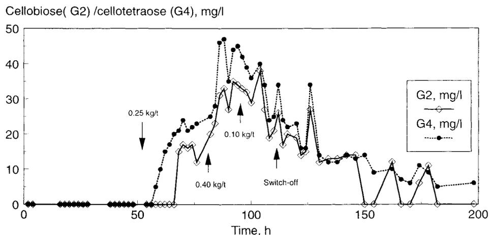
Figure 3. Concentrations of cellobiose (G2) and cello-tetraose (G4) in the white water samples taken from the bow screen during the first mill trial.
