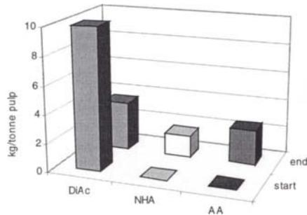
**Figure 6.** Diac hydrolysis to NHA and subsequent laccase-catalyzed oxidation to acetanilide during upflow and downflow tower operations in pilot plant. AA - acetanilide.
