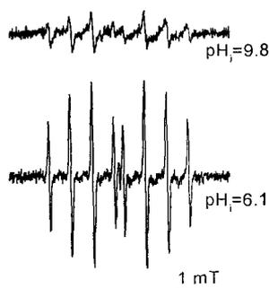
Figure 6. ESR spectra obtained with copper/ 4-AP/ H<sub>2</sub>O<sub>2</sub> with the spin trap DEPMPO at pH 9.8 and 6.1.
