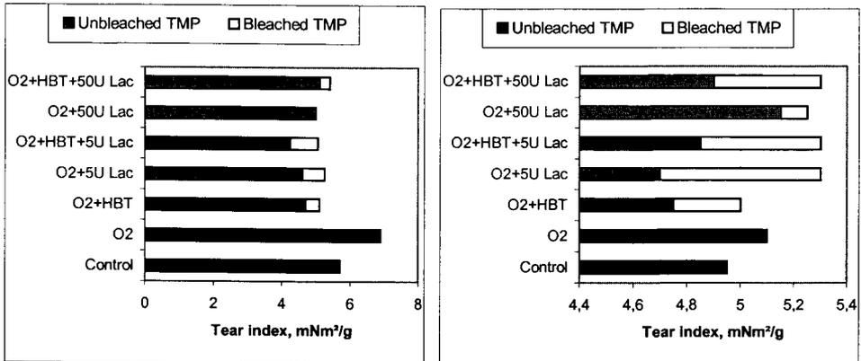
Figure 2. Evolution of tear index after different treatments with laccases applied on primary-refined (left) or secondary-refined (right) softwood TMP at 90 ml CSF.
