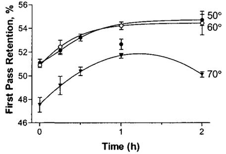
Figure 6. Effect of temperature on mannanase kinetics. Headbox stock was treated with 5 mannanase U/L of Gamanase. FPR was measured with no retention aid, and a 70 mesh screen. Data are means of 3 replicates ± standard errors.
