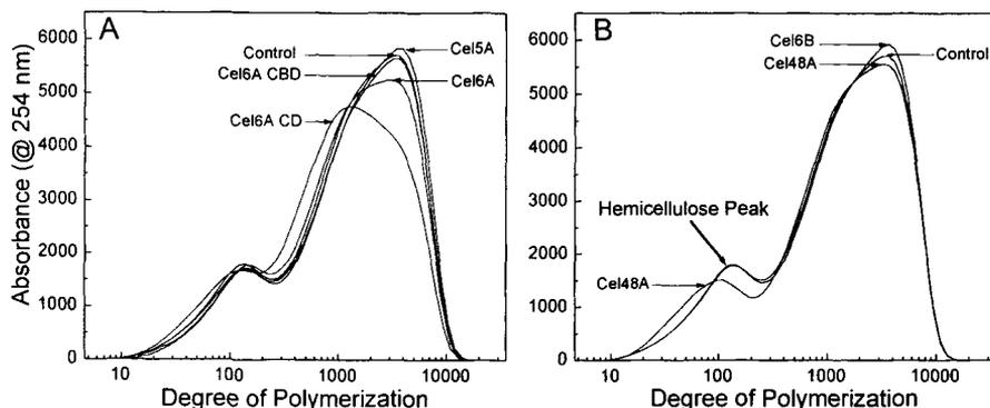
**Figure 5.** Degree of polymerisation of cellulase-treated kraft pulps.
