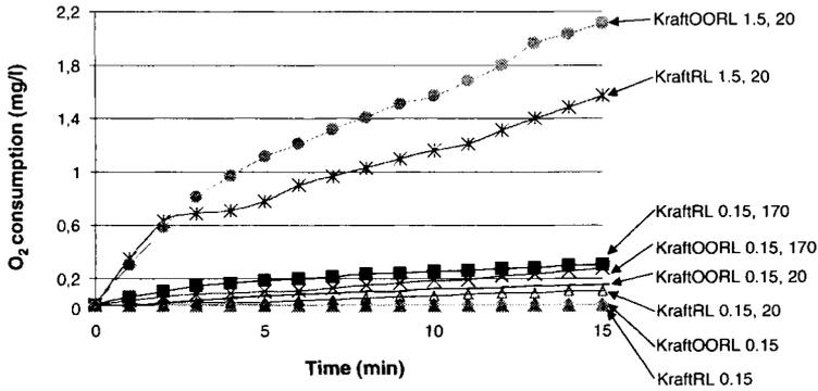
Figure 1. The reactivity of KraftRL and KraftOORL as a function of time, lignin concentration (0.15 and 1.5mg/ml) and laccase charge (20 and 170 nkat/mg).
