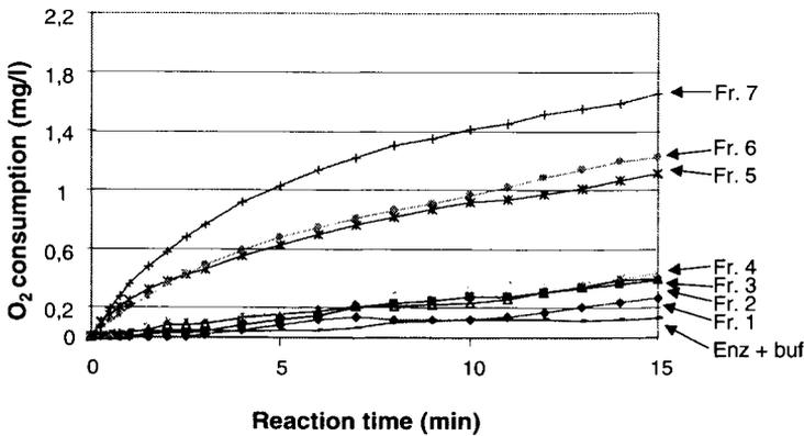
Figure 6. The reactivity of fractionated KraftRL in laccase treatments. Lignin concentration 0.13 mg/ml, laccase charge 170 nkat/mg.
