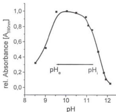
Figure 4. pH course of relative concentration of the copper coordinated to 4-AP. The arrow indicates the change of pH during a typical Cu-stage.
