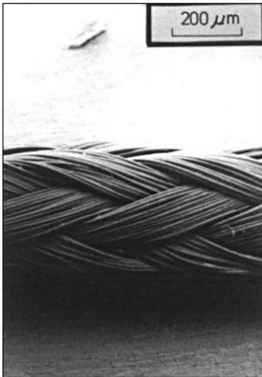
Figure 1 SEM finding of chitin braided fibers.
