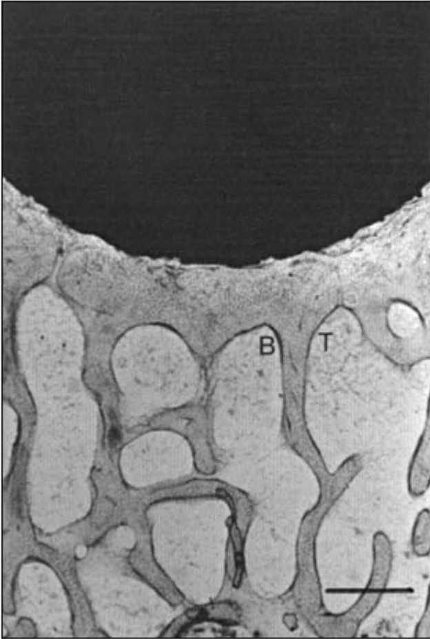
Figure 5 Distal interface of a Ti cylinder, 50µm, with part of the bony frame and perpendicularly arranged trabeculae with respect to the implant surface between bony frame and spongy bone next to the cartilage of the knee joint. Trabeculae below bony frame showing surface profiles resembling Baud' s curves (46). Trabecular surface profiles follow rules of avoiding notch stresses and having minimized weight. Note different profiles for tension (T) and bending (B). LM, Giemsa stain, bar 500 µm.
