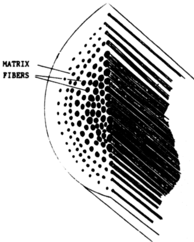
Figure 2 Schematic representing the self-reinforced composition technique by Törmälä and co-workers 1,2. The fibers function as a scaffold for the matrix substance of the same origin.
