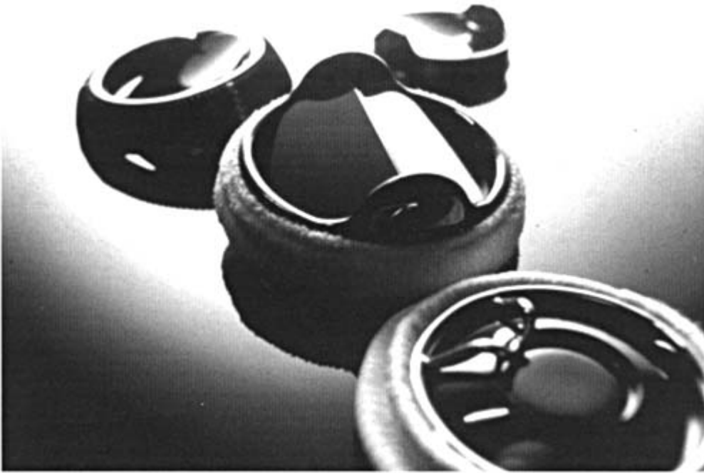
Figure 4 Pyrolytic carbon mechanical heart valve of the St. Jude design. A carbon to carbon articulation is present which shows no wear under physiologic loading of nearly 40 million cycles per year.
