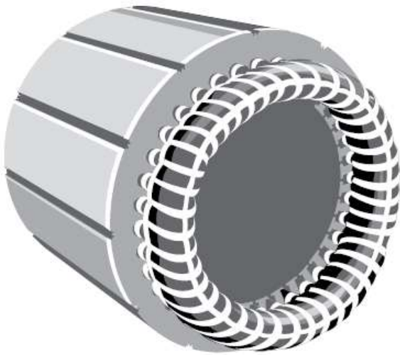
Fig.4. stator coils or winding completed
