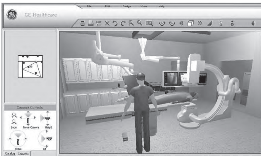
FIGURE 8-1 Example of a component-based simulation of an operating room, allowing the owners and designers to compare different equipment.
