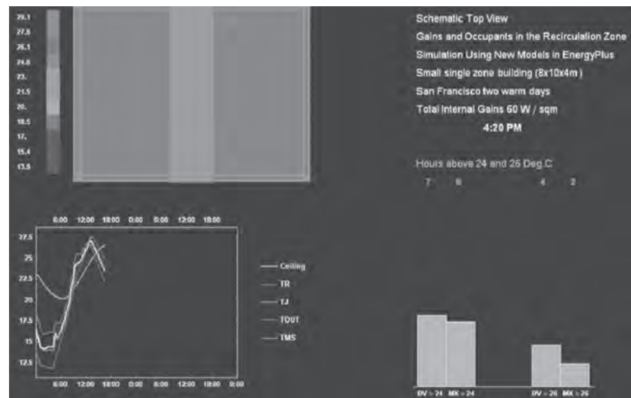
FIGURE 9-5-6 Results of an EnergyPlus simulation of a single zone office building using the new UCSD displacement ventilation model.
