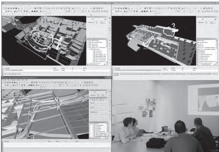
FIGURE 9-10-6 Multiple images of layout conflicts caught in the bi-weekly review meetings, using NavisWorks. Images courtesy of H3.
