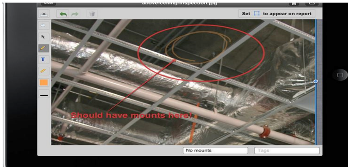
Figure 6.7: A tablet computer system displaying a quality inspection carried out to high level services
