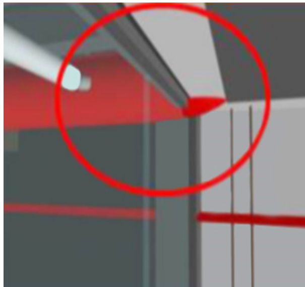
Figure 6.5: Detailed view of the detected clash between the steelwork elements
