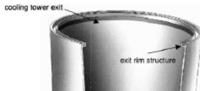
Figure 17: Stabilizing structure at the inner rim side.
