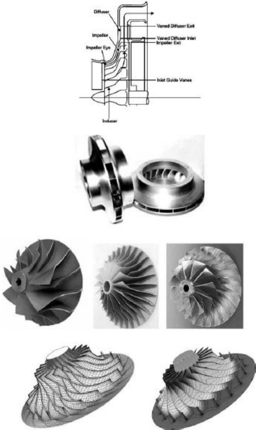
Figure 2: Examples of centrifugal impellers and modeling.
