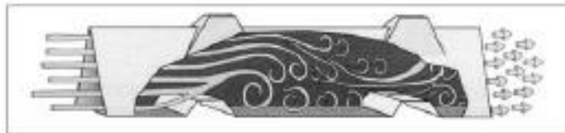
Figure 26: Conjectured flow pattern in a duct with bumps.
