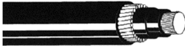
Figure 2.1 Single-core PVC/SWA/PVC cable
