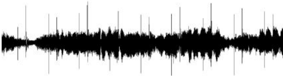
Figure 13.1 The profile of a transient noise pulse from a scratched gramophone record.
