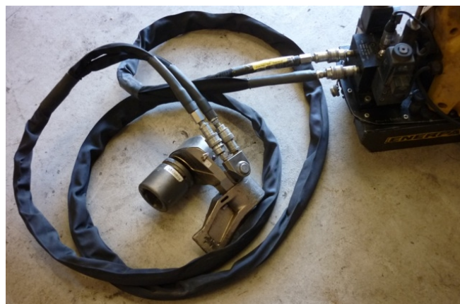
Image 3: Anti-abrasion/diffusion cover Photo from MMG century mine innovation award (2011) – See further information.
