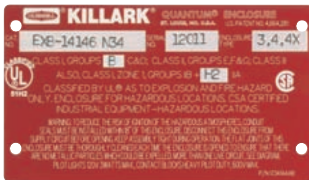
Killark North American nameplate example for explosionproof and dust-ignitionproof enclosure showing listing for Class I, Div. 1, Class II, Div. 1, Class III and Class I Zone 1 locations.
