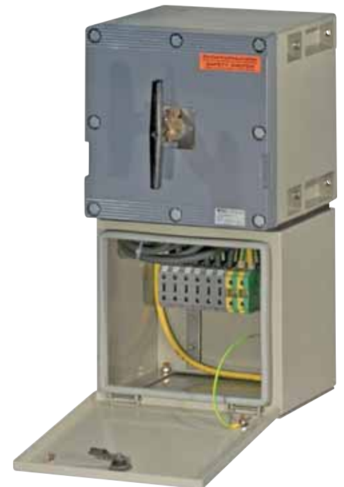
Rotary switch in flameproof enclosure of the series GHG 64 with flat joint and flanged-on Ex-e connection box for indirect connection
