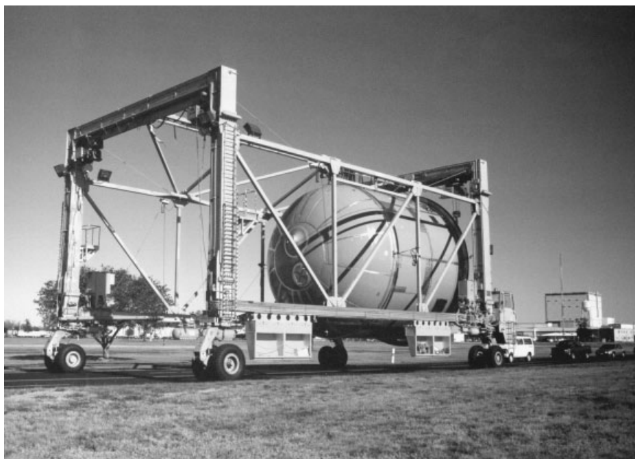
Figure 5 Fuel tanks and booster rockets such as those of the Space Shuttle are 2xxx alloys, originally 2219 and 2419, now Al–Li “Weldalite” alloy 2195.
