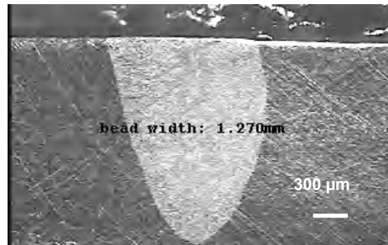
Figure 6.7. Macrograph of butt joint bead profile
