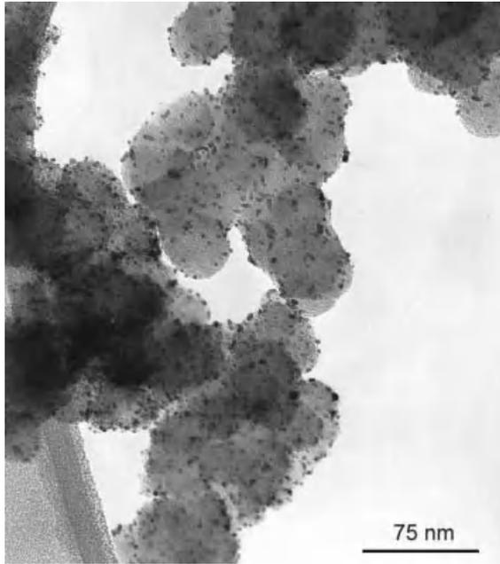
**Figure 5.5** Electron microscope image of some fuel cell catalyst. The black specks are the catalyst particles finely divided over larger carbon supporting particles. (Reproduced by kind permission of Johnson Matthey plc.)
