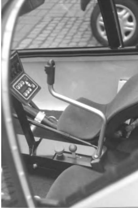
**Figure 10.5** Stick controller fitted to a vehicle
