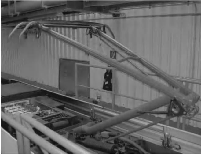
**Figure 4.4** Overhead pantograph. (Source: [http://en.wikipedia.org/wiki/Pantograph\\_\(rail\)](http://en.wikipedia.org/wiki/Pantograph_(rail)).)
