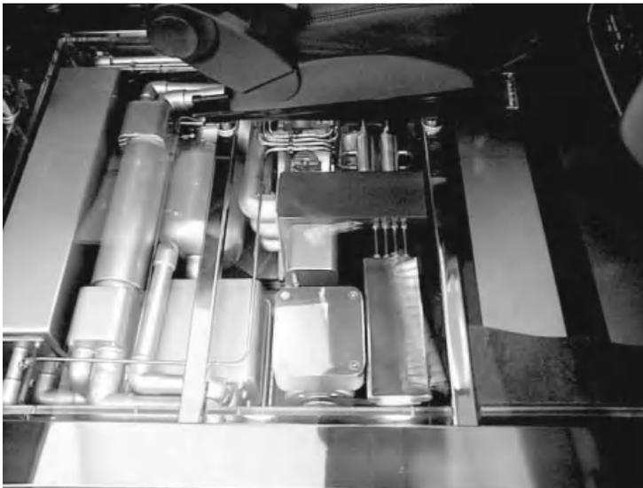
**Figure 6.6** Packaging of the Nekar 5 methanol fuel processor
