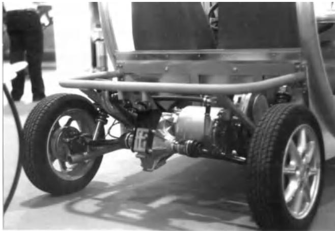
**Figure 9.7** Example of type (a) of Figure 9.6 on an experimental electric vehicle by MES-DES SA. The mounting of the motor is transverse, so there is no drive shaft
