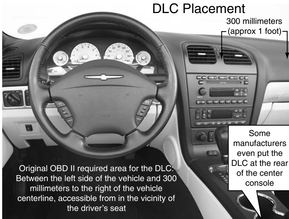
Figure 8-6 Original OBD II DLC location requirement. © Cengage Learning 2012
