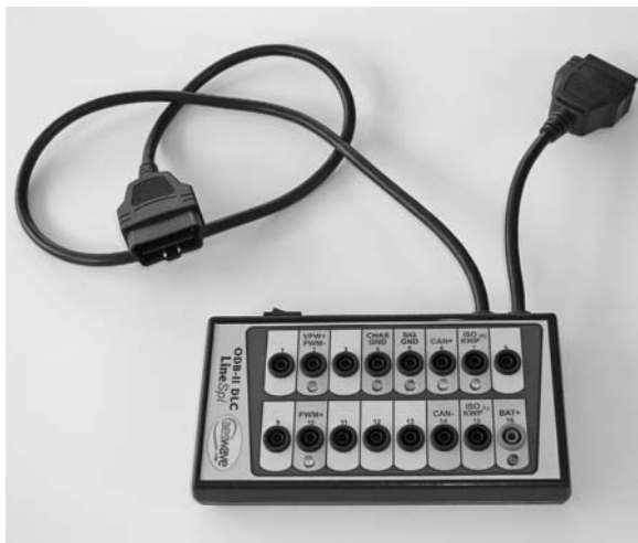
Figure 6-4 DLC breakout box. © Cengage Learning 2012
