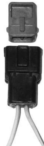
Figure 12–68 SPOUT connector with shorting bar, 1986 and newer. © Cengage Learning 2012
