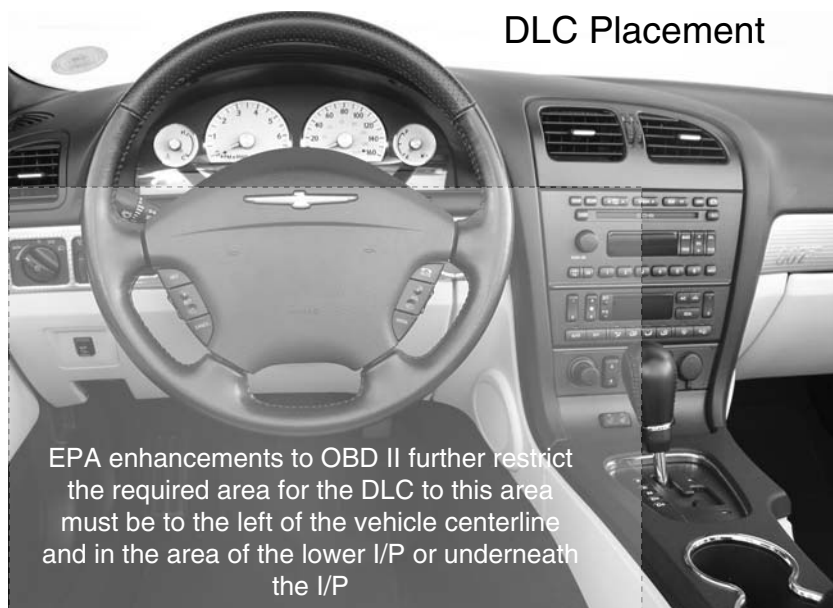
Figure 8-7 OBD II DLC location as enhanced by the EPA. © Cengage Learning 2012
