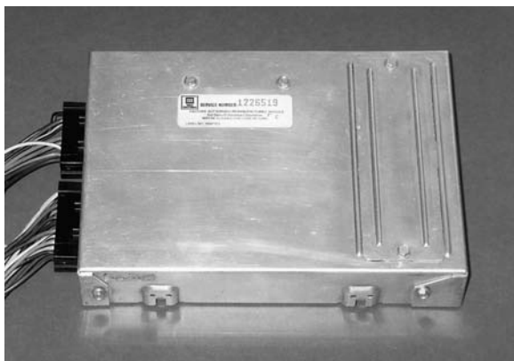
Figure 10–1 GM's Computer Command Control system PCM. © Cengage Learning 2012
