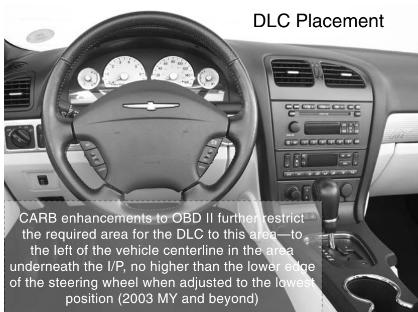
Figure 8-8 OBD II DLC location as enhanced by CARB. © Cengage Learning 2012
