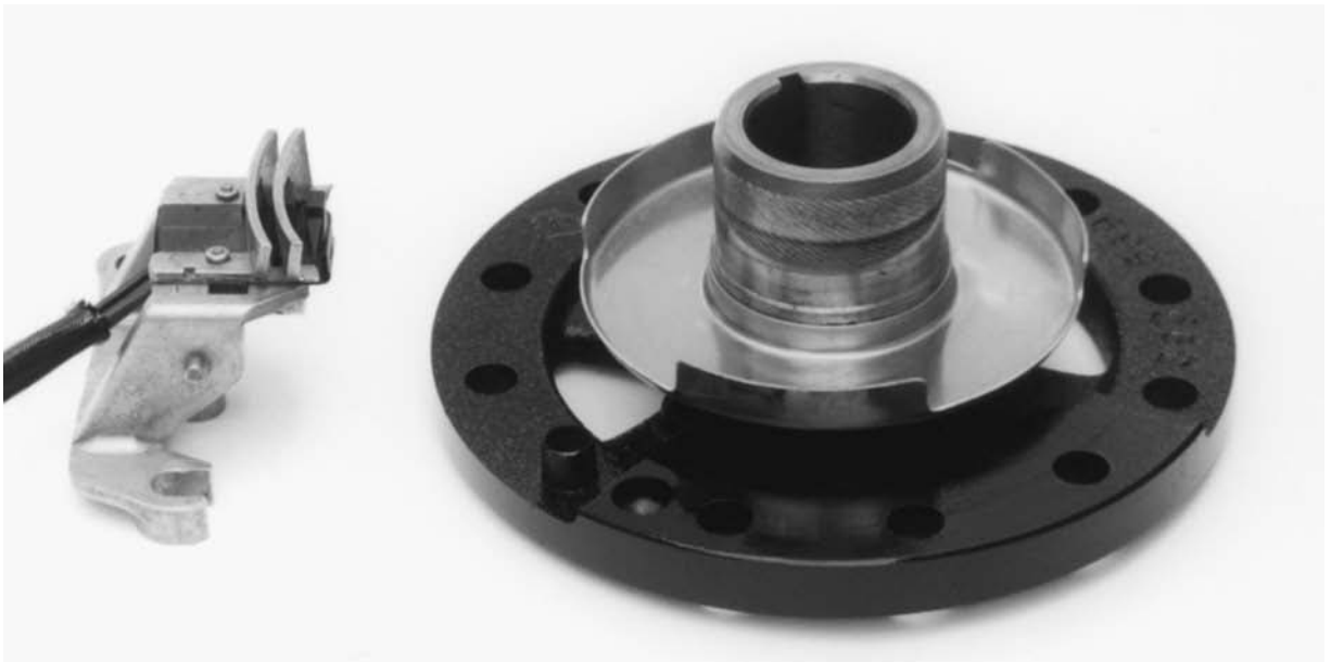
Figure 10-47 Hall effect crankshaft sensor and harmonic balancer with three vanes and three windows.
