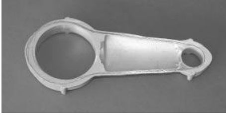
Figure 11.1 Section of a textile-reinforced aluminum piston rod. Especially, the locally anisotropic mechanical properties of the material and of the entire component are in the focus of this test case scenario. Anisotropic permeabilities relevant to the production of this component by investment casting are investigated as well.
