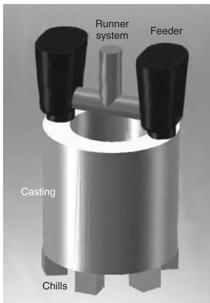
Figure 12.5 Calculation domain consisting of the actual casting, the feeders, the runner system, the chills, and the mold. Mold and FDM cell structure are omitted for clarity reasons.
