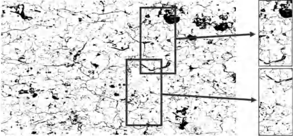
Figure 5.9 Segmented SEM image of the APS coating (porosity = 25.4%) and two extracted RVEs with maximal and minimal porosities.
