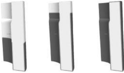
Figure 12.3 Immersion of the quarter model into the water bath: symmetry surfaces and surfaces covered by air are light gray, immersed surfaces are dark gray.
