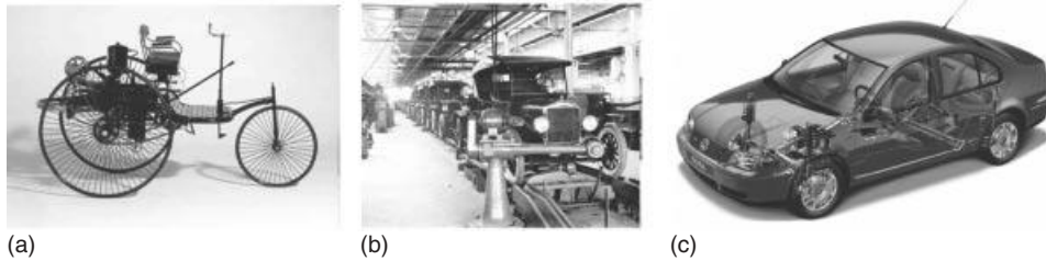
Figure 2.1 Platform concept in production of cars. (a) Manufacture of an individual car does not need any standardization (image by Daimler AG). (b) Standardized cars can be produced much quicker and
