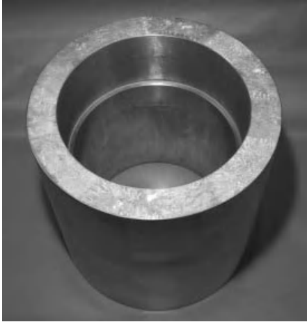
Figure 12.1 Bearing housing made from highly alloyed stainless steel.
