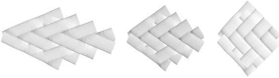
Figure 11.10 Braid structures being generated using WiseTex on the basis of different geometrical data for braid angles (angle between roving and withdrawal direction of mandrel) of 20, 30, and 45°.
