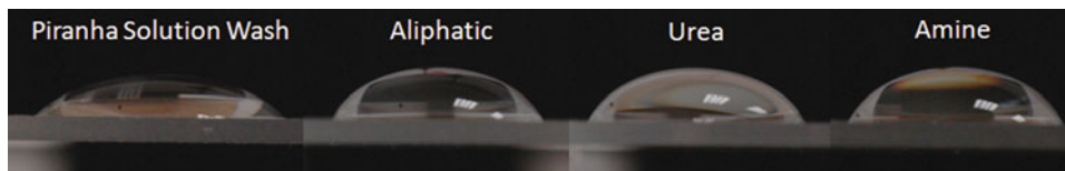
Fig. 4.2 Water droplet contact angles on the surface treated glass slides
