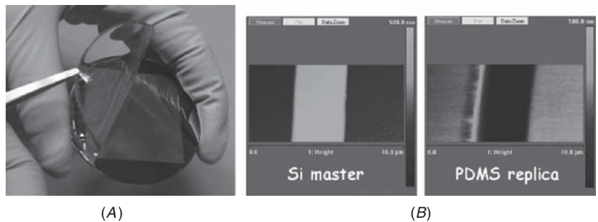
FIGURE 5.5 PDMS stamps for soft lithography: (A) peel off, (B) AFM images of silicon, and PDMS structure reproduction. Copyright © IEEE 2008.
