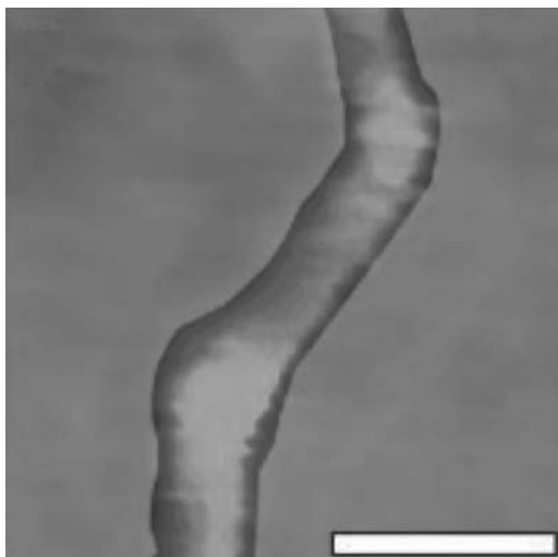
FIGURE 12.12 QD made using two kinks created by AFM manipulation (scale bar is 25 nm). 57
