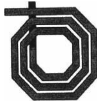
Fig. 3.31 An example of a flat-coil inductor suitable for integration on chips [© 3.36]. (Copyright © IEEE. Reproduced with permission.)
