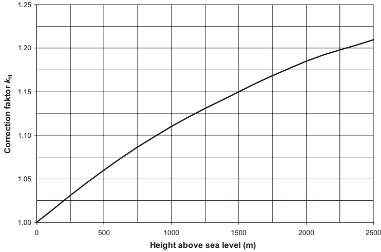
Figure 9.4 Correction factor for global radiation on a normal (horizontal) surface: influence of geographical height above sea level.
