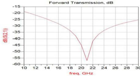
Fig. 15. Variation of isolation with frequency for new CPW obtained from Agilent ADS
