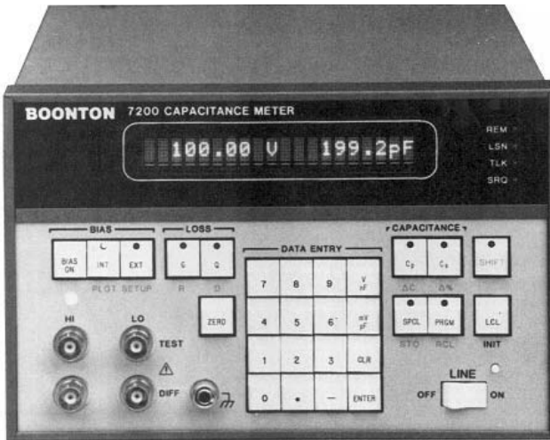
Figure 4.6. The front panel of a capacitance–voltage meter showing a measured value of 199.2 pF at a diode bias of 100 V. This instrument can measure both conductance (charge flow in phase with the voltage) and capacitance (charge flow 90° behind the voltage).
