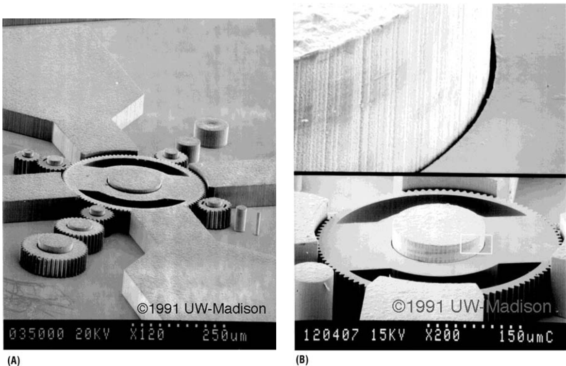
Figure 19.35 (A) Assembled Ni structures for friction and magnetic properties testing. (B) Assembled shaft-gear combination made from Ni with a height of 150 \mu\text{m} . The bushing tolerance is 0.25 \mu\text{m} (from Guckel [75], © 1998 IEEE).
