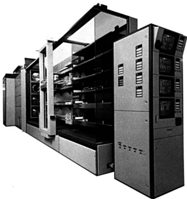
Figure 4.24 Horizontal tube oxidation/diffusion system includes computer controller, load station, and four tubes (photo courtesy of ASM International).
