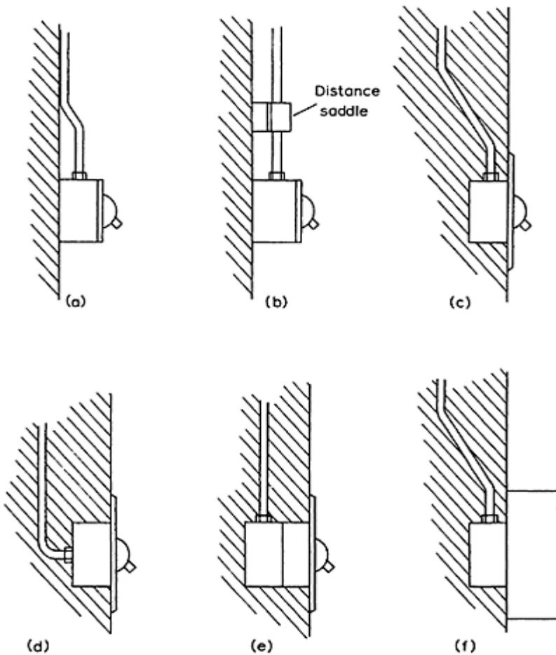
*Figure 3.9* Conduit entries to equipment
