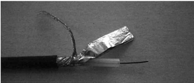
*Figure 2.10* Coaxial cable
