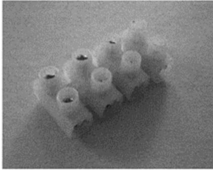
*Figure 1.21* Connector block
