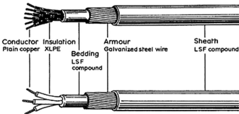
*Figure 2.9* LSF cable (Courtesy of B.I.C.C)
