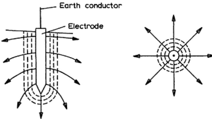
*Figure 9.21* Current from electrode into earth
