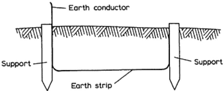
*Figure 9.20* Copper strip electrode
