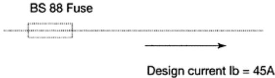
Figure 4.1 Device rating related to design current
