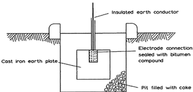
Figure 9.19 Cast iron plate electrode
