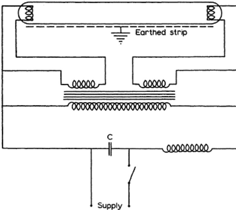
*Figure 7.4* Quick-start circuit
