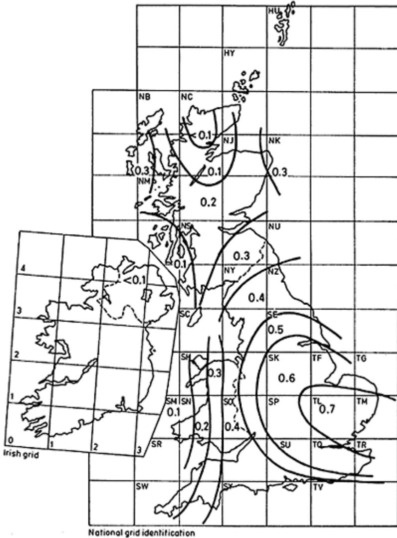
Figure 14.5 Number of lightning flashes to the ground per km<sup>2</sup> per year for the UK
