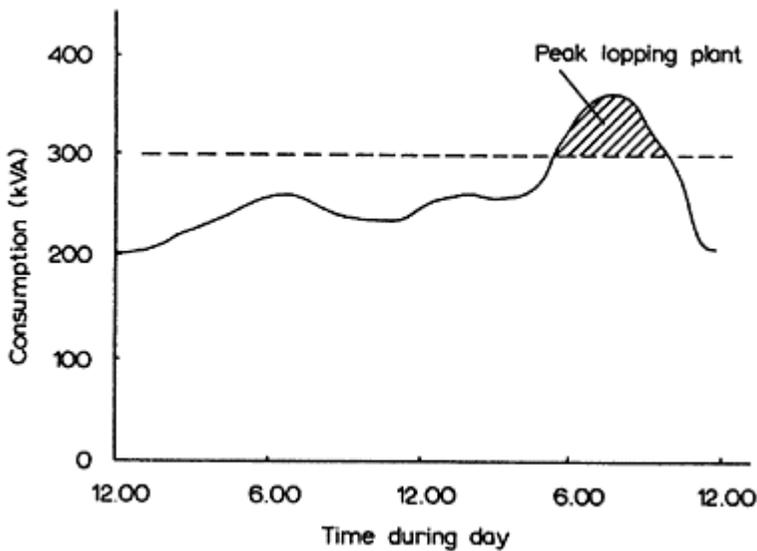
*Figure 15.3* Load diagram
