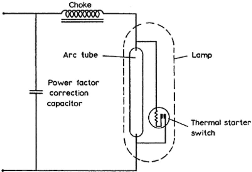
Figure 7.9 Typical solarcolour lamp circuit
