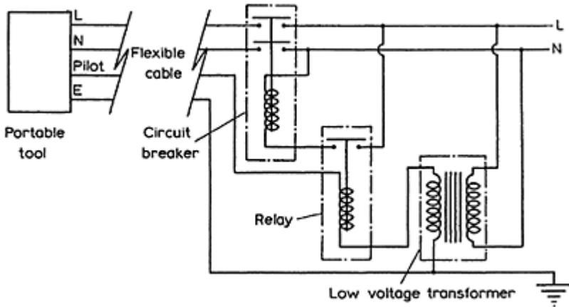
*Figure 9.17* Monitored earth leakage protection
