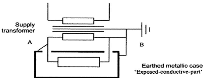
Figure 9.1 Earth fault
