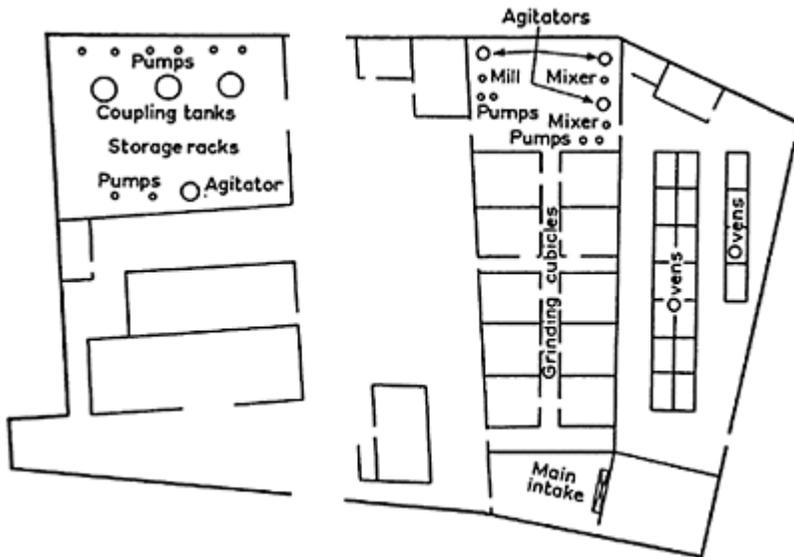
Figure 18.4 Factory ground-floor equipment layout
