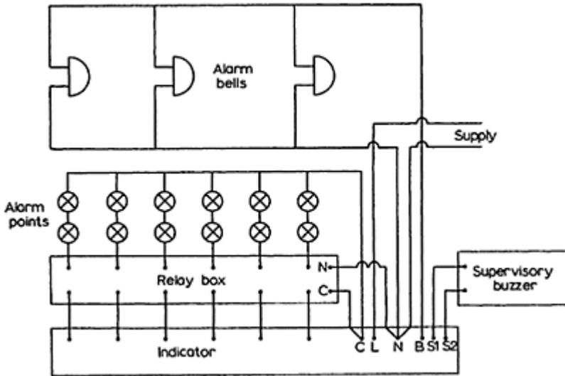
Figure 10.4 Fire alarm with indicator
