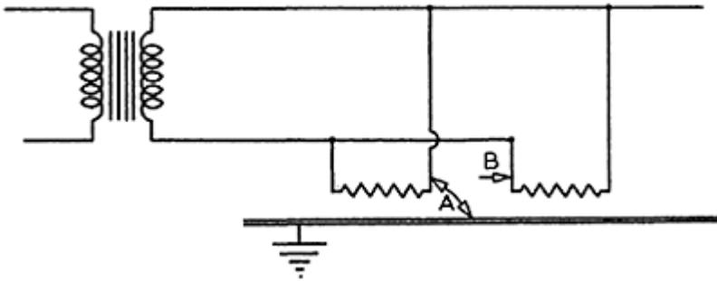
*Figure 9.11* Wrong use of isolating transformer
