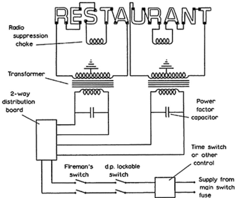
Figure 7.13 Circuit for display lighting
