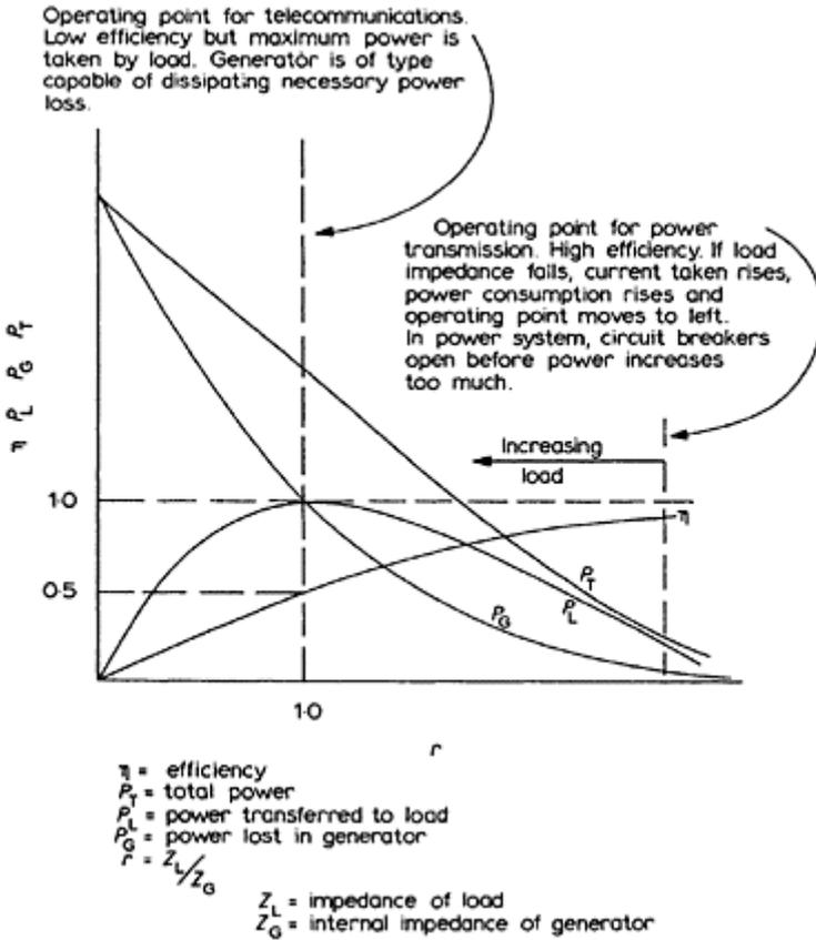
Figure 13.9 Operating points of transmission lines
