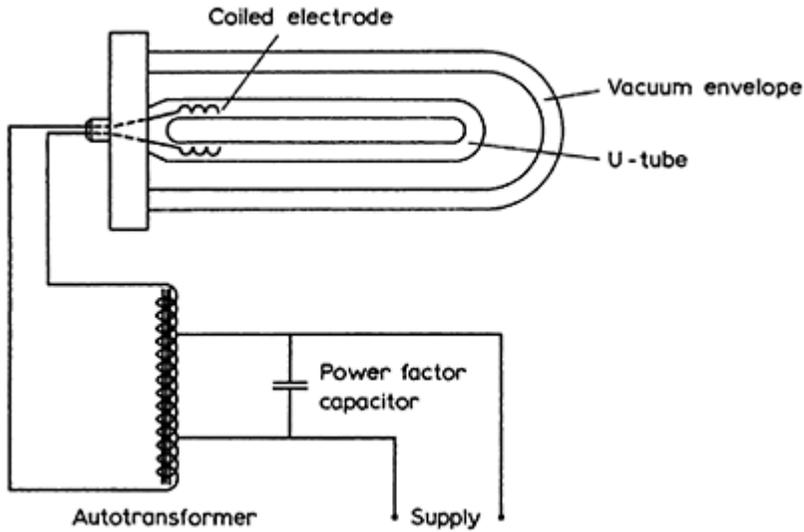
*Figure 7.8* Sodium discharge lamp
