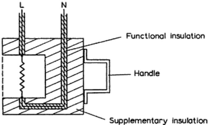
*Figure 9.24* Double insulation
