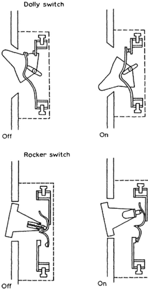
*Figure 1.2* Switch mechanisms
