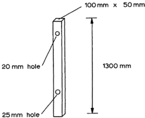
*Figure 3.6* Bending block
