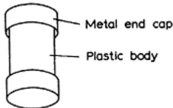
*Figure 9.3* Cartridge fuse
