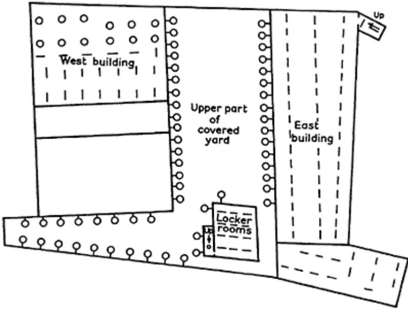
Figure 18.2 Factory first-floor lighting layout
