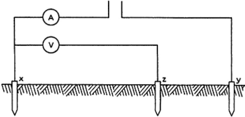
*Figure 9.23* Earth electrode resistance test
