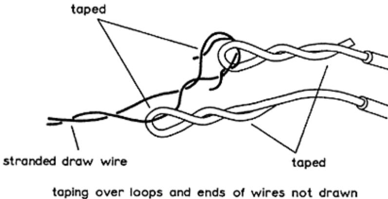
*Figure 3.11* Connection of cable to draw cable
