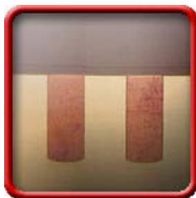
Fig. 7.8 Copper-filled via-hole. Reprinted with the permission of Allvia Inc. ( www.allvia.com )
