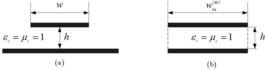
Fig. 2.7 Air-filled microstrip (a) and its parallel-plate model (b)
