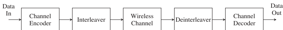
Figure 8.1 System block diagram illustrating the use of interleaving and deinterleaving in a wireless data communication system.
