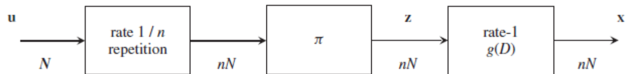
Figure 10.4 Encoder for an (nN, N) RA code. The numbers below the input–output lines indicate the size of the corresponding binary vectors.
