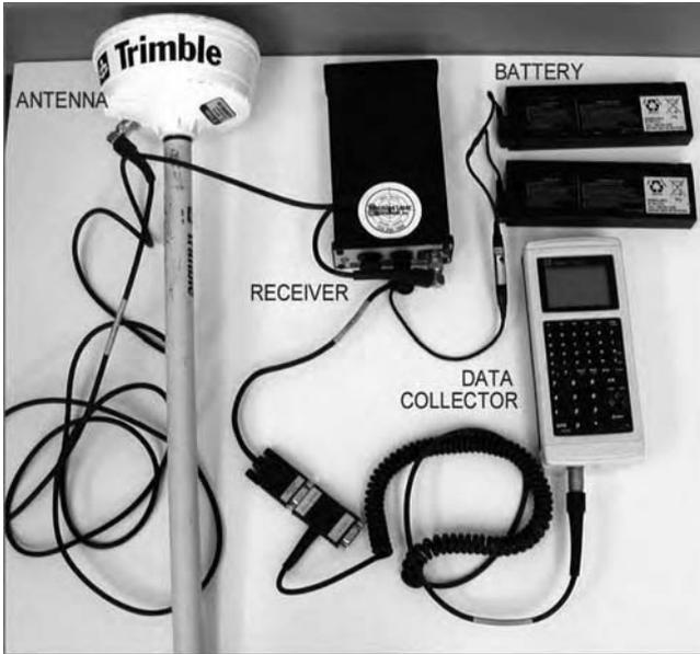
**Figure 5.3** Components of Trimble Pathfinder Pro XR Backpack.
