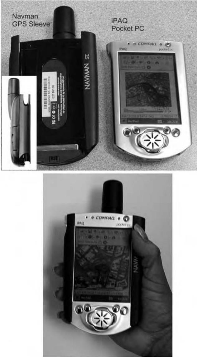
**Figure 7.3** Sample mobile GIS device. Above: Navman GPS sleeve and iPAQ Pocket PC shown separately; below: iPAQ inserted into the sleeve.
