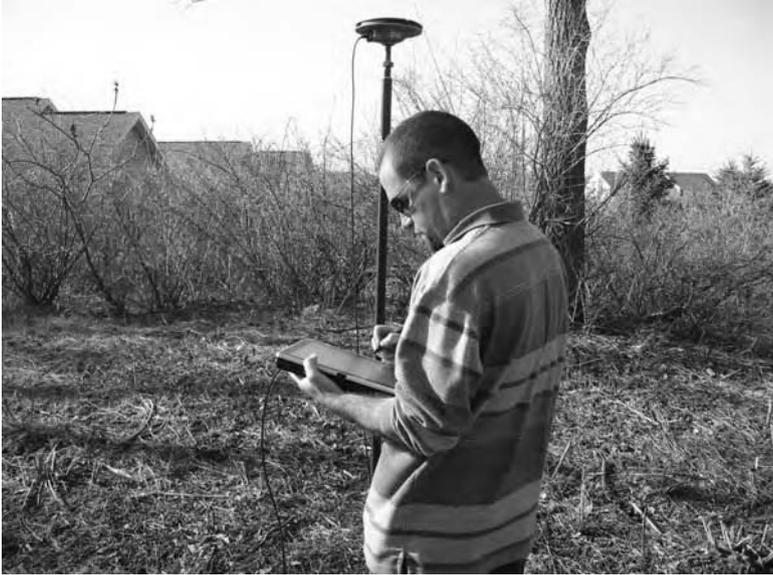
**Figure 7.1** Tablet PC being used for GPS and field data collection.
