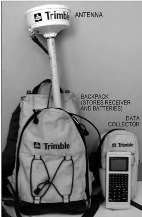
**Figure 5.2** Advanced GPS equipment example (Trimble Pathfinder Pro XR Backpack).
