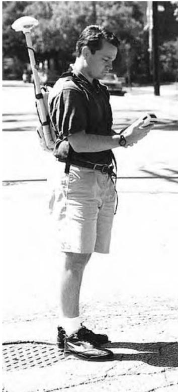
GIS data collection for sewer system manholes using GPS.
