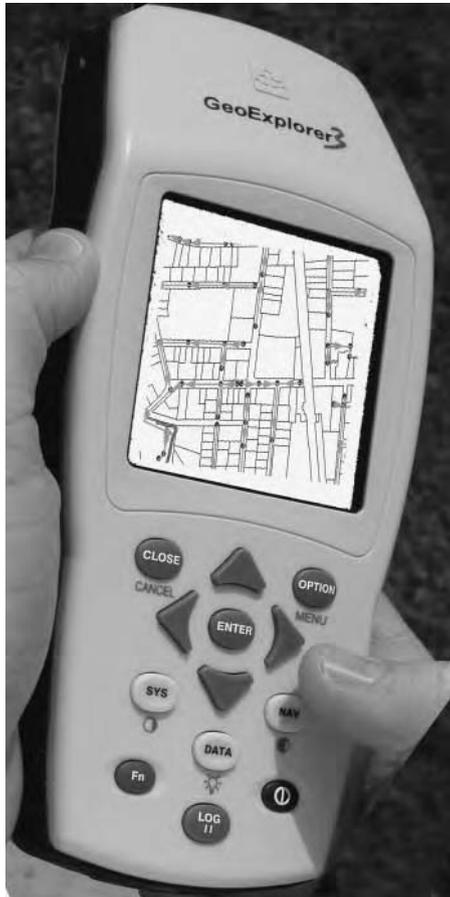
**Figure 5.1** Basic GPS equipment example (Trimble Geoexplorer III).
