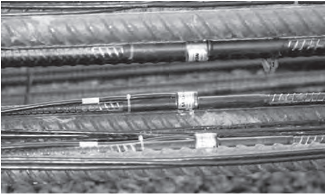
Figure 9.21 Vibrating wire strain gauge installation. (Photograph courtesy of PMC Limited, Durham.)
