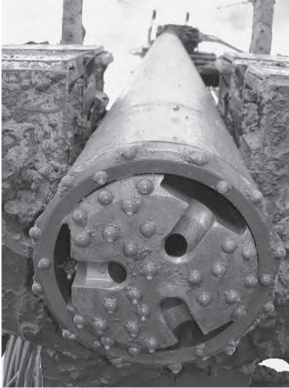
Figure 3.15 Down-hole hammer bit. (Photograph courtesy of Ritchies.)
