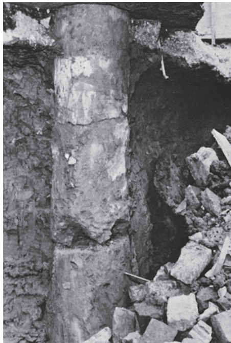
Figure 7.16 The consequence of 'topping-up' after extraction of casing. (Photograph courtesy of CIRIA, London.)
