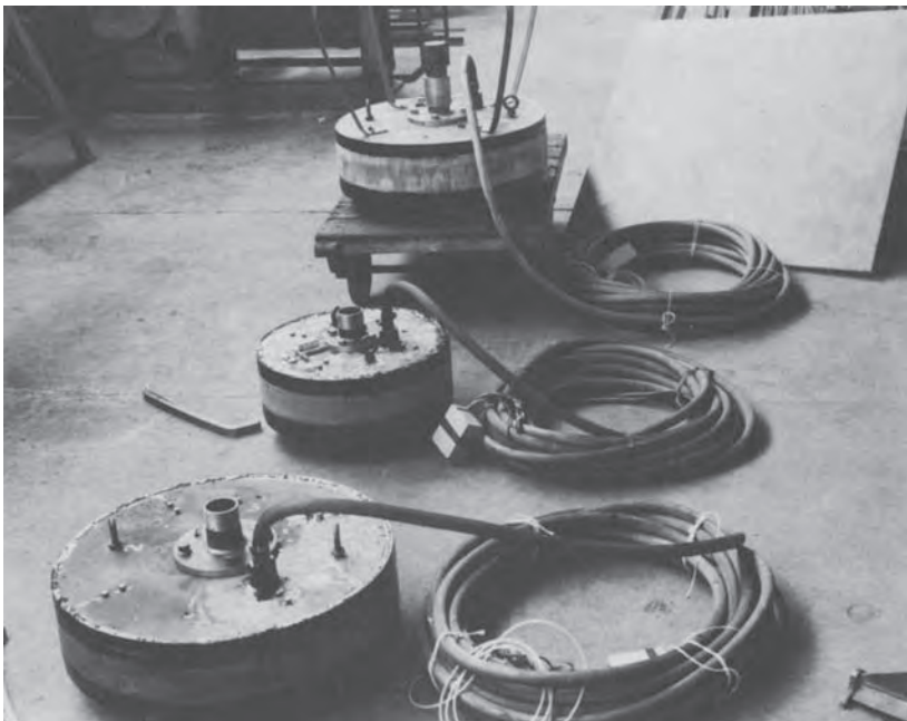
Figure 9.19 BRE pile load cells. (Building Research Establishment: reproduced by permission of the Controller, HMSO. Crown copyright.)
