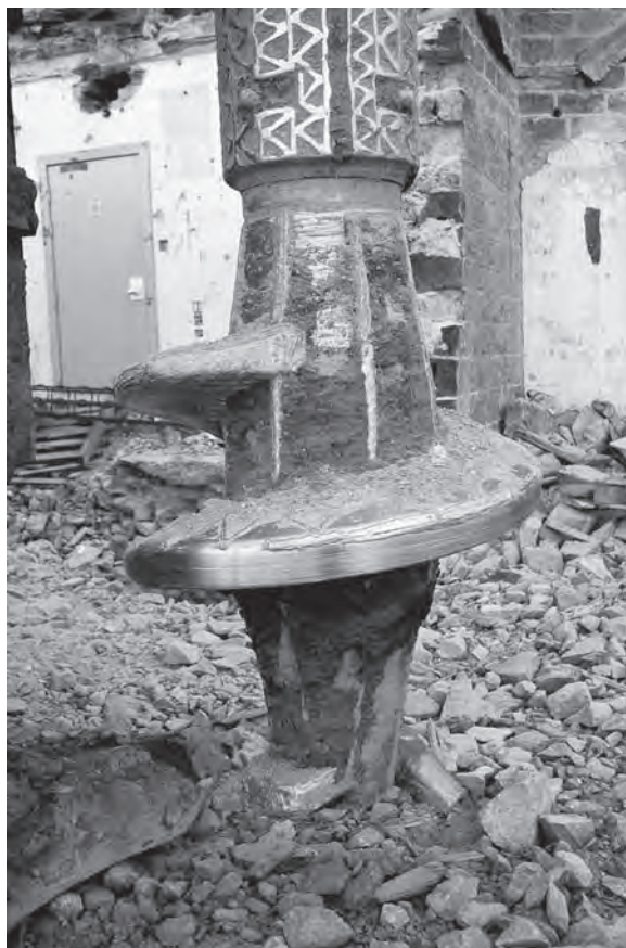
Figure 3.9 CHD pile auger head. (Photograph courtesy of Roger Bullivant Limited.)
