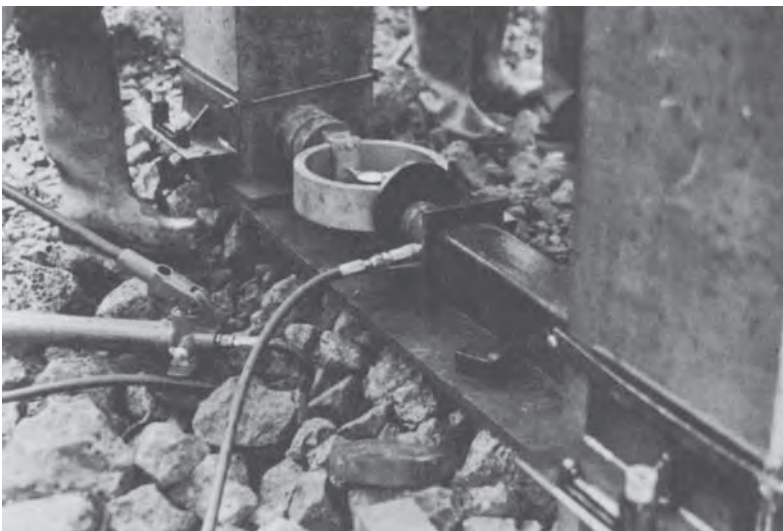
Figure 9.27 Lateral pile load test. (Photograph courtesy of Westpile Ltd., Uxbridge.)
