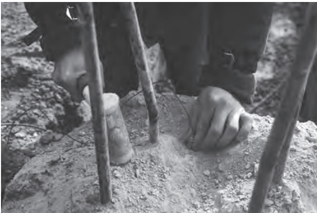
Figure 8.5 Seismic integrity test (sonic echo method) in operation.
