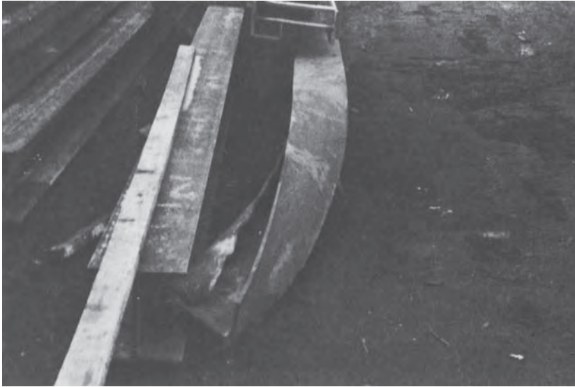
Figure 7.3 Buckling of steel H-pile driven into boulder clay. (Photograph courtesy of Sir Robert McAlpine & Sons Ltd.)
