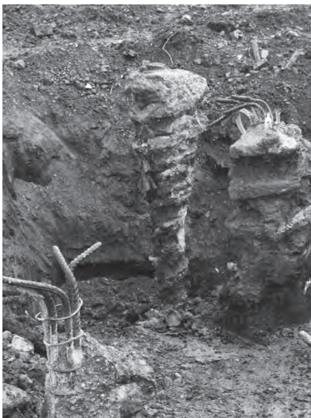
Figure 7.24 Necking of a screw pile shaft likely to have been the result of poor control of extraction rate of the auger.
