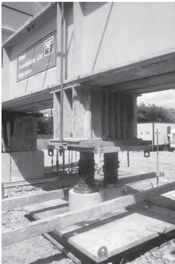
Figure 9.6 Details of load train. (Photograph courtesy of Sir Robert McAlpine & Sons Ltd, London.)
