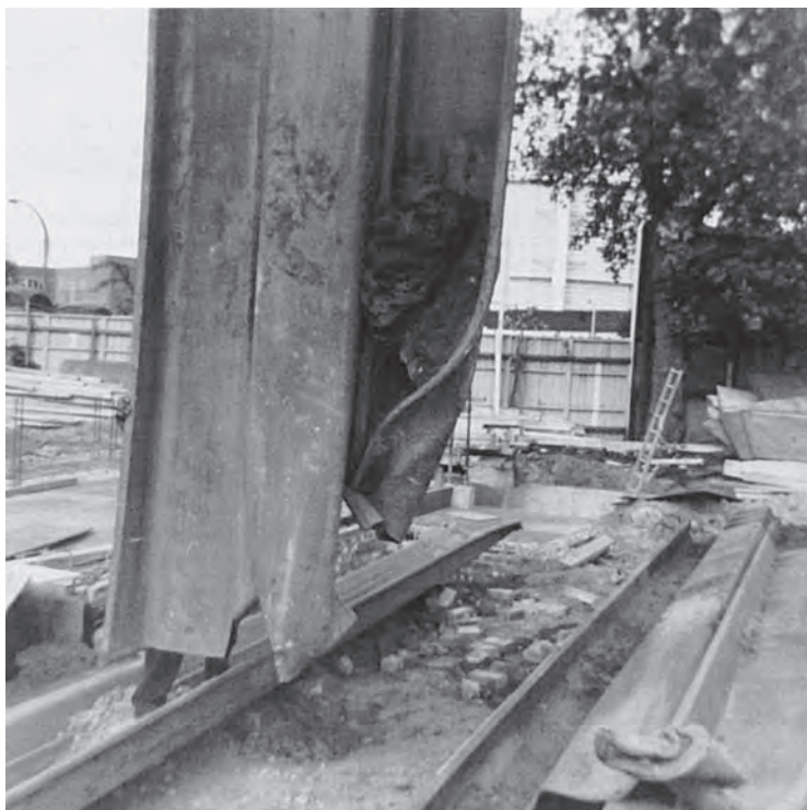
Figure 7.2 Buckling of sheet steel piling. (Photograph courtesy of CIRIA, London.)
