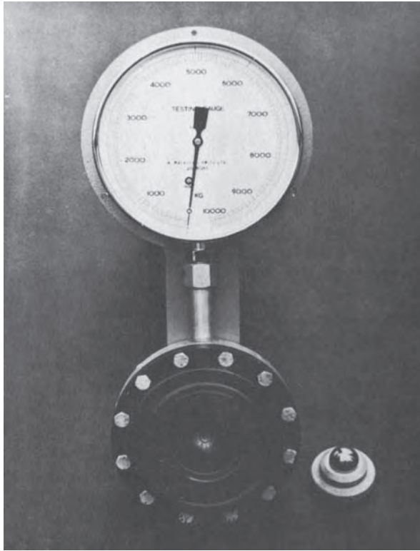
Figure 9.8 Hydraulic load capsule. (Photograph courtesy of A. Macklow-Smith Ltd., Camberley.)
