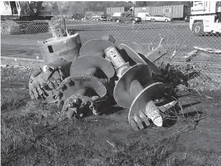
Figure 3.18 Boring tools used in the construction of rotary bored cast-in-place piles. Foreground – heavy duty augers, background-drilling buckets. (Photograph courtesy of Carillion Piling.)
