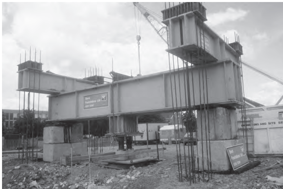
Figure 9.2 A 2500-tonne pile load test using tension piles to provide reaction. (Photograph courtesy of Cementation Piling and Foundations Ltd., Rickmansworth.)
