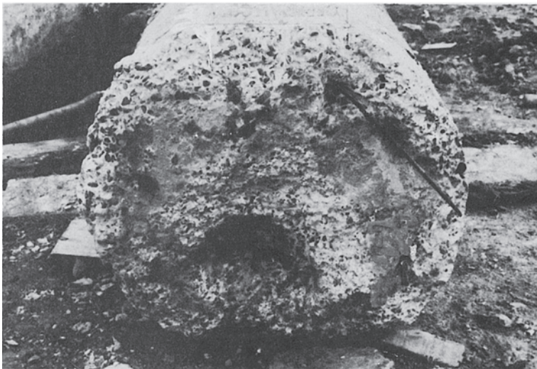
Figure 7.8 Toe of small-diameter pile filled with silt prior to concreting. (Photographs courtesy of CIRIA, London.)
