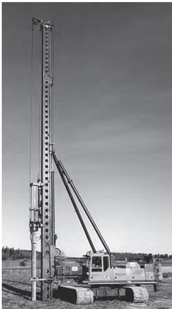
Figure 3.10 Banut 850 piling rig, crawler-mounted, hydraulically operated machine with forward, backward and side-to-side raking facilities. Overall height of rig 25 m. (Photograph courtesy of Banut.)
