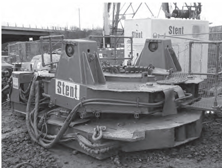
Figure 3.23 Casagrande hydraulic casing oscillator with diesel powered pump.
