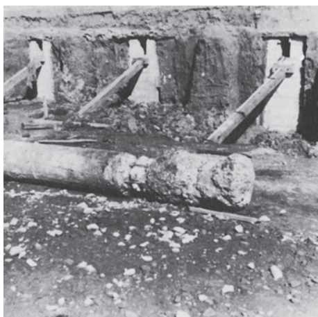
Figure 7.9 Toe of pile after concreting with water in bore. (Photograph courtesy of CIRIA, London.)
