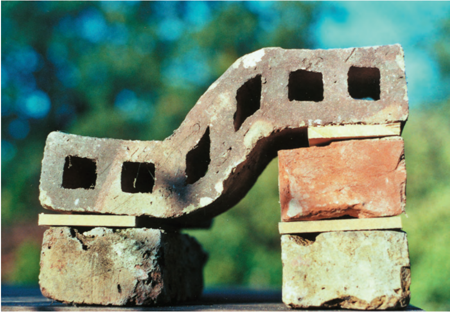
Fig. 4.3 The Victorians used special-shaped bricks as wall ties in their cavity walls.
