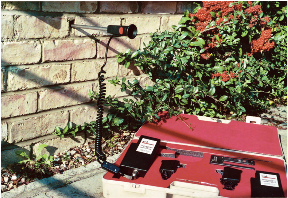
Fig. 1.2 Borescope for inspecting inside wall cavities, sub-floor voids and other areas. The wide-angle lens provides good depth of field.
