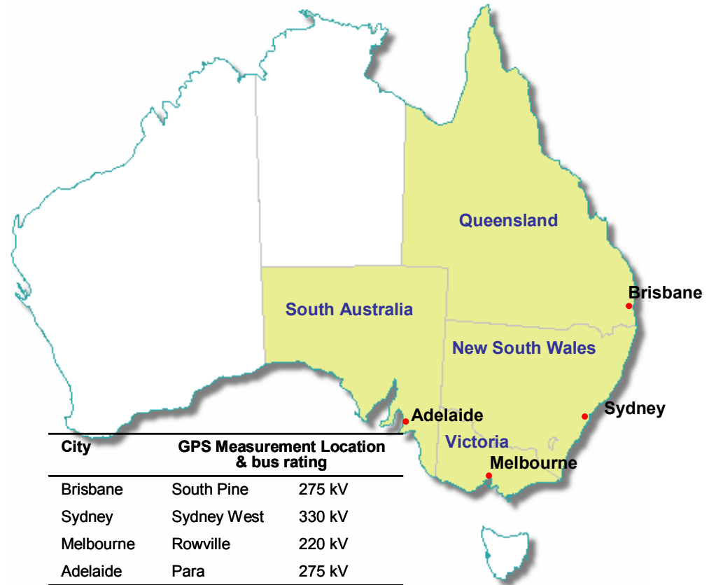
Figure 1-1 States associated with the eastern Australian large interconnected power system (shaded). State capital cities that represent generation nodes and measurement site location and ratings are shown.
