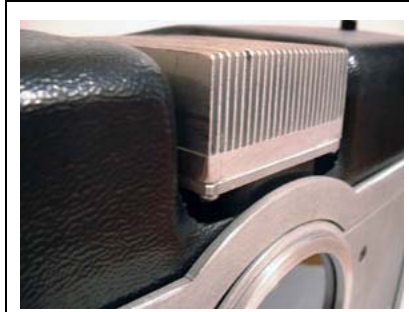
Figure 1: Heat Sink of Kinkajou Alpha Prototype.
