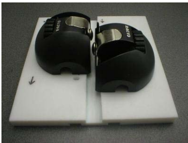
Figure 2: Microfilm Trimmer. Using mat-cutters, 16mm microfilm is cut down 1/8” so it fits on standard VHS spools.
