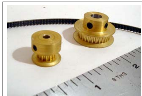
Figure 27: Timing Belt and Timing-Belt Pulleys.
