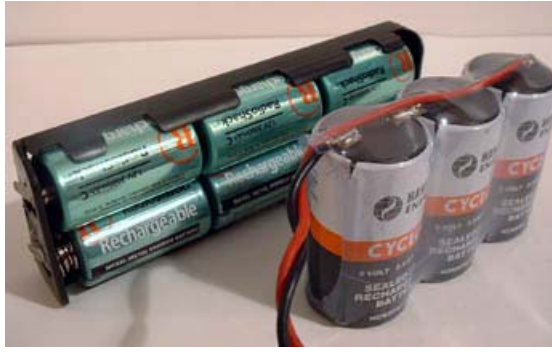
Figure 14: Old and New Battery Packs. The new three-cell Lead-acid pack (foreground) costs less than a third as much and will provide more than twice the life of the six Ni-MH C cells (back) used in the Kinkajou alpha prototype.
