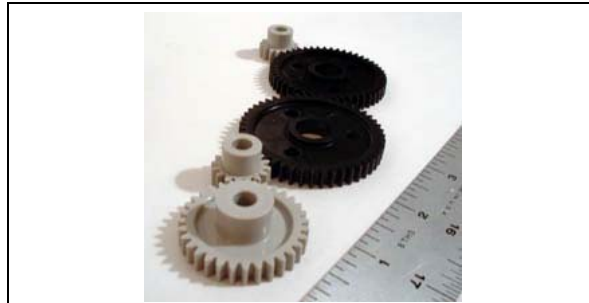
Figure 34: Plastic Gears. These gears can be used as part of an indexing system.
