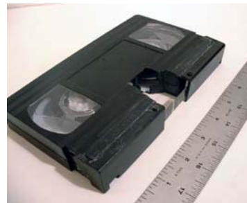
Figure 3: Modified VHS Cassette. The cassette has a hole cut in it so the microfilm can interface with the optics unit.
