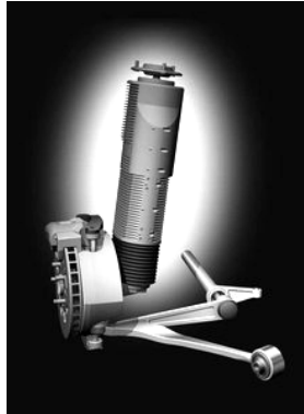
Fig. 5.54 Semi-active E-M ABW AWA suspension (with the linear E-M motors) that is termed ' Bose® suspension ': front corners contain E-M uprights and custom lower control arms [EISENSTEIN 2005; LOTUS 2005].
