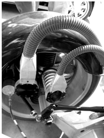
Fig. 5.151 The active wheel (AW) technology uses a traction E-M motor to turn the wheel and all active ABW AWA suspension components within the wheel and tyre [Larry Edsall/Special to the Detroit News; EDSALL 2004].
