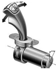
Fig. 4.8 Principle layout of a unique sidestick (joystick) [DAIMLERCHRYSLER 2004].
