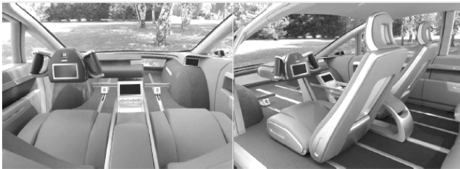
Fig. 4.7 Miniature colour screen and two handgrips [GM Opel's Hy-Wire FC HEV; THIESEN, 2003; SCHMIDT, 2004]
