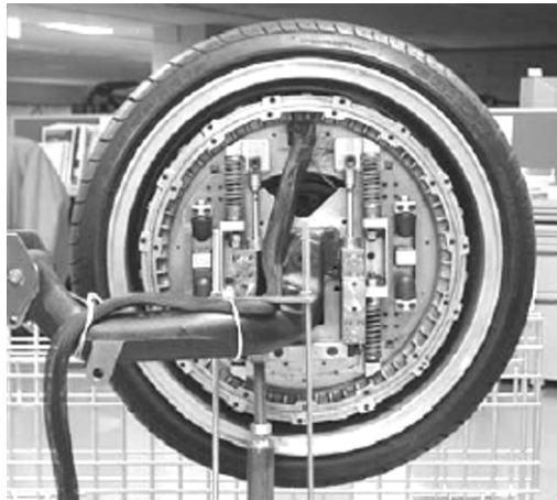
Fig. 5.153 Dynamic-absorbing steered, motorized and/or generatorised wheel (SM&GW) [Bridgestone Corporation; BRIDGESTONE 2003].
