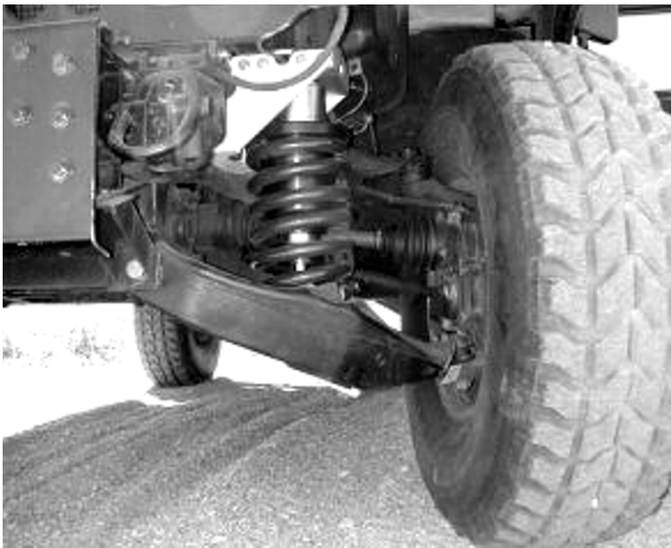
Fig. 5.48 HMMWV SOADS mechatronic control system [MILLENWORKS 2005A].
