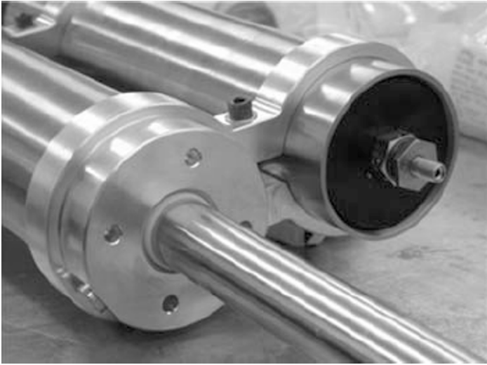
Fig. 5.76 Stryker 8-wheeled, 20-Mg infantry carrier vehicle's MR shock absorber [RMSV; RMSV 2004].
