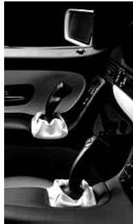
Fig. 4.11 The SBW vehicle may be accelerated by lightly pushing forward compact joysticks that are linked electronically [DAIMLERCHRYSLER 2004].
