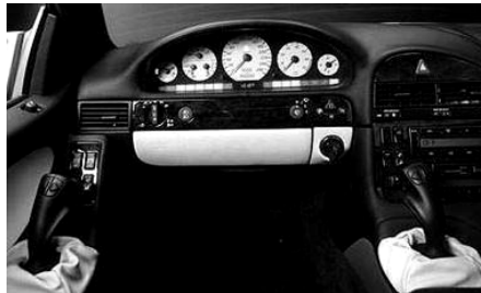
Fig. 4.12 View of the sidesticks' comfortable location [DAIMLERCHRYSLER 2004].
