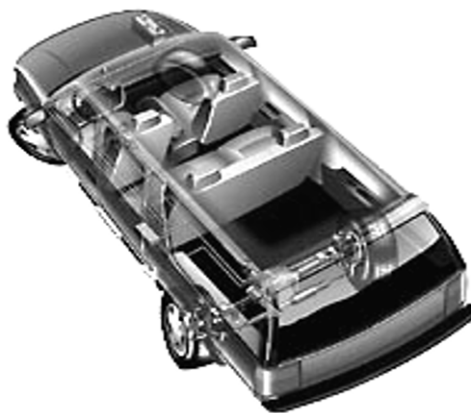
Fig. 4.98 Half-truck equipped with the SBW 4WS conversion mechatronic control system [Delphi 'QUADRASTEER' TM ].
