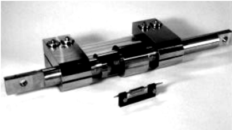
Fig. 5.167 Outlook of three E-M-M actuators to create a linear stepper E-M-M motor [Energen Inc.; JOSHI 2000].
