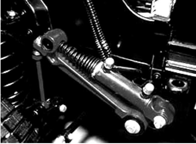
Fig. 5.107 Active cornering enhancement (ACE) [Ford Motor Company; BRAUER 1999; MEMMER 1999].
