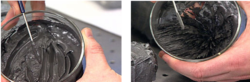
Fig. 5.58 Oily fluid full of tiny iron particles before being near a magnet (above); and after [MIT Hatsopoulos Microfluids Lab.; GILBERT AND JACKSON 2002].
