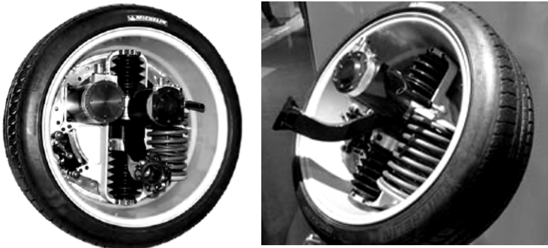
Fig. 5.150 The Michelin Concept vehicle can lean thanks to its active AW ABW AWA suspension [Challenge Bibendum in Shanghai; MEILLAUD 2005].
