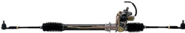
Fig. 4.43 Fluidical power steering (FPS) – vehicle velocity responsive type [Hitachi Co.; HITACHI 2004].
