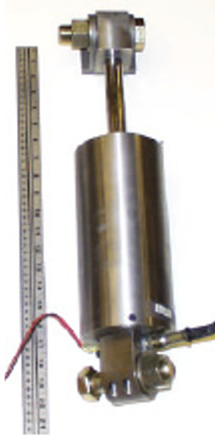
Fig. 5.75 HMMWV's MR shock absorber [U.S. Army Research Office; LIU ET AL. 2004].
