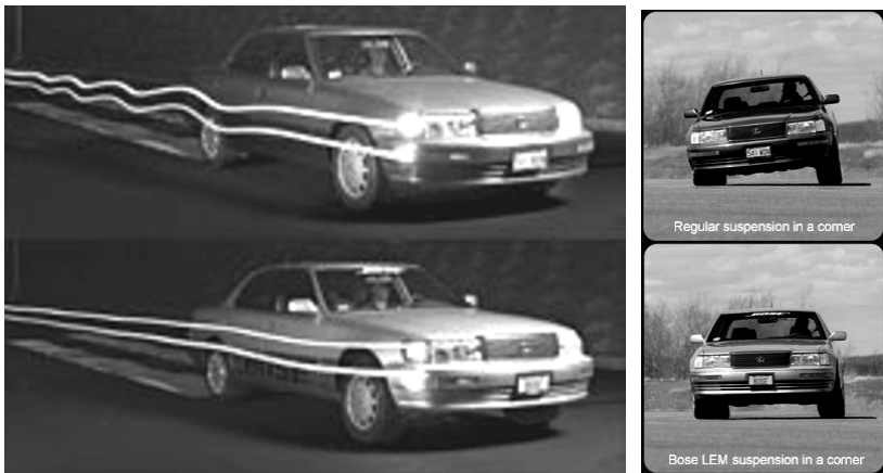
Fig. 5.146 The active E-M ABW AWA suspension-equipped automotive vehicle (below) has far better vehicle-body control than the standard automotive vehicle (above) [AKA Bose Corporation Headquarters, Framingham, Massachusetts, USA; JENNINGS 2005].
