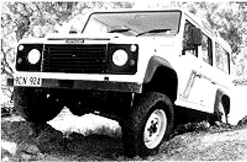
Fig. 5.13 Kinetic™ suspension-equipped two-wheel-drive (2WD) vehicle can perform a conventionally equipped four-wheel-drive (4WD) vehicle [Tenneco Automotive].
