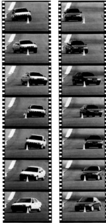
Fig. 5.131 Comparison of a conventionally passive suspended automotive vehicle with the active F-P-M 4WA ABW suspended automotive vehicle [Citröen; CITROËN 2001].
