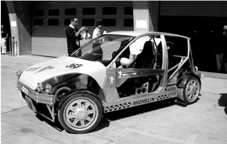
Fig. 5.152 The Michelin concept vehicle is equipped with the tyre maker's active wheel (AW) technology that packages the active ABW AWA suspension mechatronic control system inside the wheels [Larry Edsall/Special to the Detroit News; EDSALL 2004].
