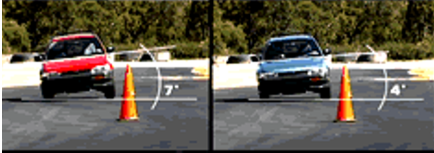
Fig. 5.19 Comparison of two the same passenger automotive vehicles: Shubaru Imprezza with the conventional passive suspension (red) and Kinetic™ passive (P) suspension (right) [Kinetic™ Suspension Technology; KINETIC 2005].
