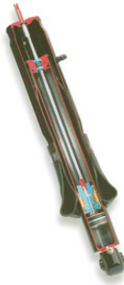
Fig. 5.67 Cutaway of the single-stage, mono-tube MR shock absorber with rear levelling provisions [General Motors Corp.; GILBERT & JACKSON 2002]
