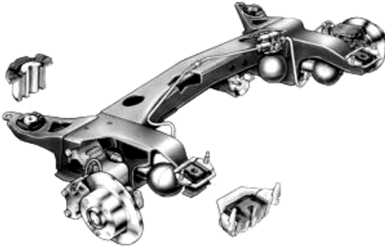
Fig. 5.126 Rear suspension [Citroën; CITROËN 2001].
