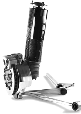
Fig. 5.145 The A E-M ABW AWA suspension (with the tubular linear E-M motors) that is termed 'Bose® active suspension' [LONGORIA 2004; McCORMICK 2004].
