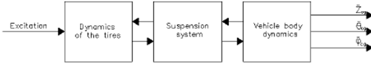
Fig. 5.5 A passive AWA suspension mechatronic control system [HYVÄRINEN 2004].
