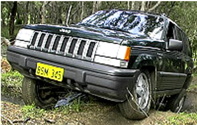
Fig. 5.15 Jeep Grand Cherokee with the Kinetic™ suspension has a free articulation limit of 55.0 cm (22 “) and an ultimate articulation limit of 77.5 cm (31 “), compared to the standard automotive vehicle’s ultimate limit of 47.5 cm (19 “) [Tenneco Automotive; BROGE 2000].
