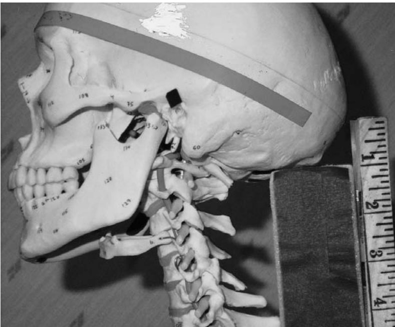
Figure 8.5 The curvature of the skull is an important determinant in hyperflexion, since an inch or two in the height of the head restraint may be critical if 'lift-up' occurs.
