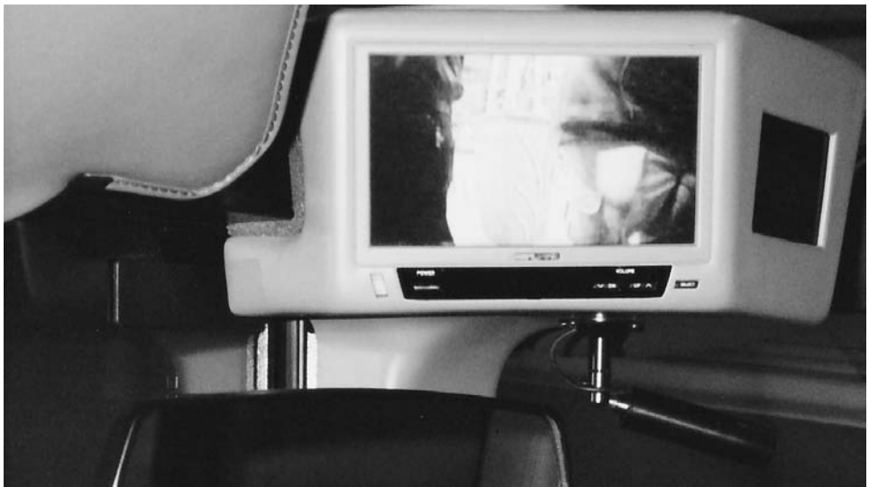
Figure 8.13 A three-way video display: one for the driver, one for the front seat occupant, and one for the rear seat passengers. It is located above the rear-view mirror. What are the occupant biokinetics with the head rotated to the right or left?
