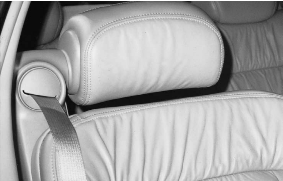
Figure 8.7 Integrated seatbelts (belts in seat) that go over the shoulder can reduce ramping (ejection to the rear compartment from reclined seats or high-yielding seats during a rear collision).
