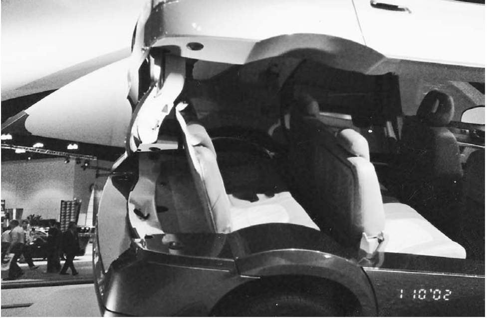
Figure 8.14 Body lifted to show the proximity of rear passenger heads to the rear window. Note the depth of the rear crush zone. With a mismatch-and-override rear collision, how does this affect occupant protection?
