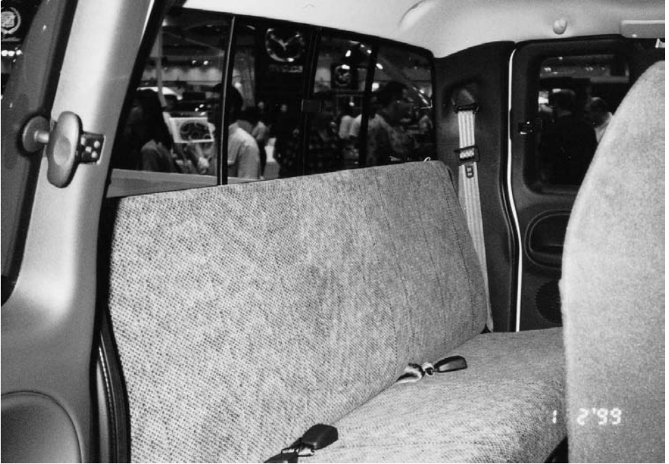
Figure 8.8 Some vehicles are sold with shoulder-height seatbacks and no head restraints.
