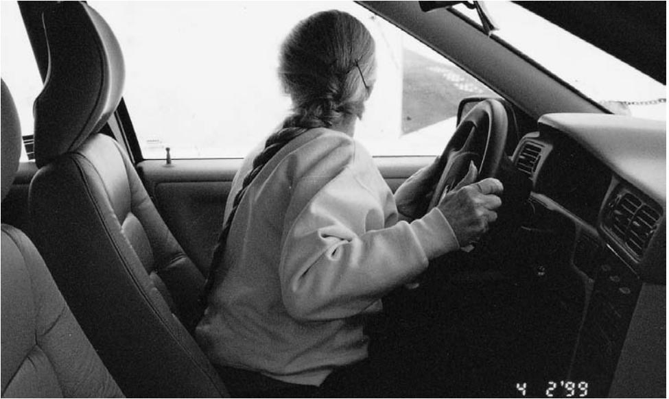
Figure 8.6 The driver may look to the rear before a lane-change maneuver in an emergency, crash-avoidance situation. As the driver tightens the arm muscles and leans forward, the chest is too close to the airbag. The use of belt pretensioners corrects this situation by pulling the upper torso back into an erect position before the airbag fires.
