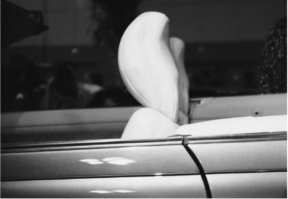
Figure 8.10 Head restraints should be about an inch (2.54 cm) from the occupant's head and reach to the top of the head.
