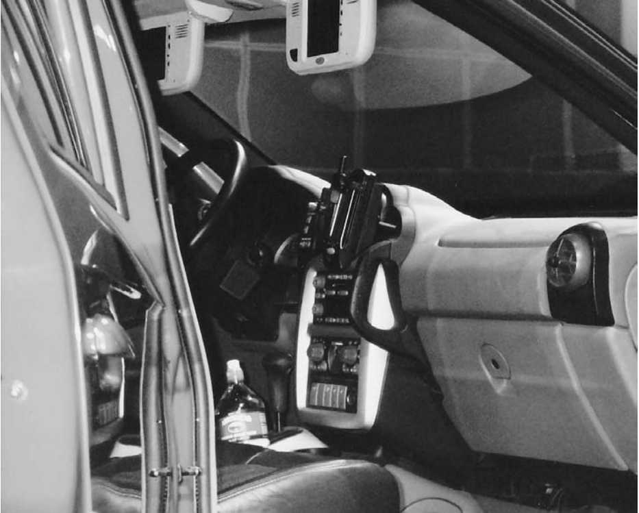
Figure 8.12 Flip-down video monitors. Some vehicles have up to seven video displays, both flip-down and inserted in the rear of the seatbacks. In terms of a collision, what does this do to crashworthiness and occupant dynamics?
