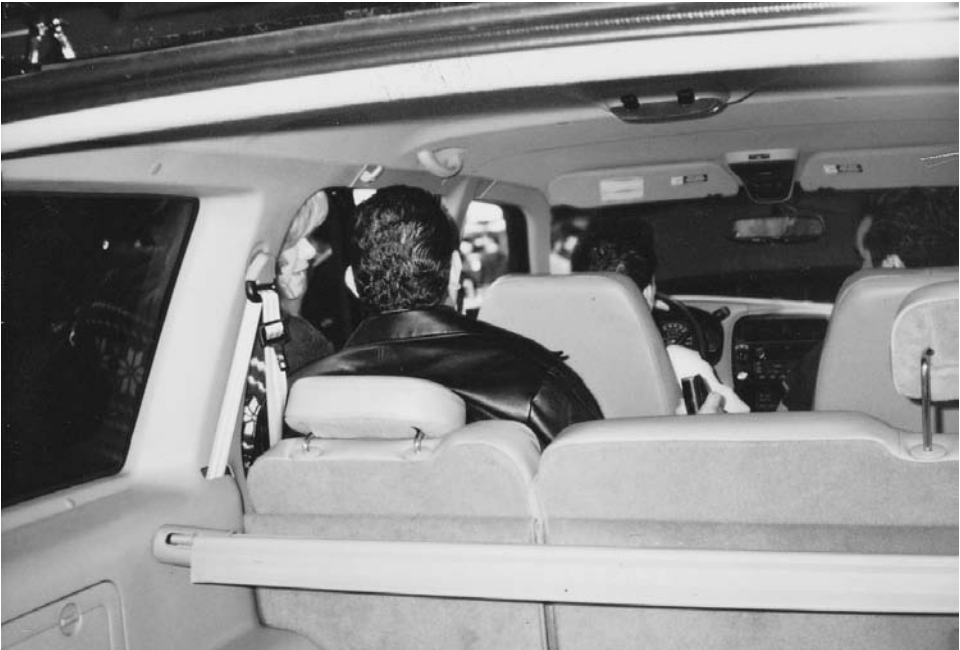
Figure 8.4 An adjustable head restraint is often left in the ‘down’ position, creating an unnecessary hazard or unsafe condition.
