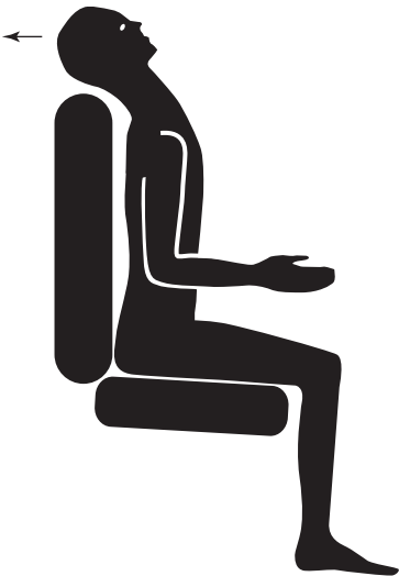
Figure 8.1 During a rear collision, a low head restraint may permit the driver's head to rotate abruptly rearward, resulting in hyperextension injuries to the neck and deceleration injuries to the brain.
