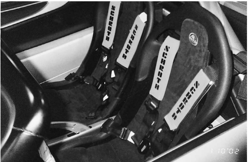
Figure 8.15 Four-point occupant restraints (two shoulder belts) have been used in specialty vehicles. Some automobiles are now scheduled for this major improvement in vehicle safety.
