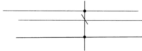
5. Run dimension lines THROUGH the wall [see above]. CAD likes to dimension just to the face of the wall, leaving a gap.
