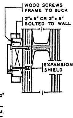
(3) Frame attached to block face scale  $1\frac{1}{2}'' = 1'-0''$
