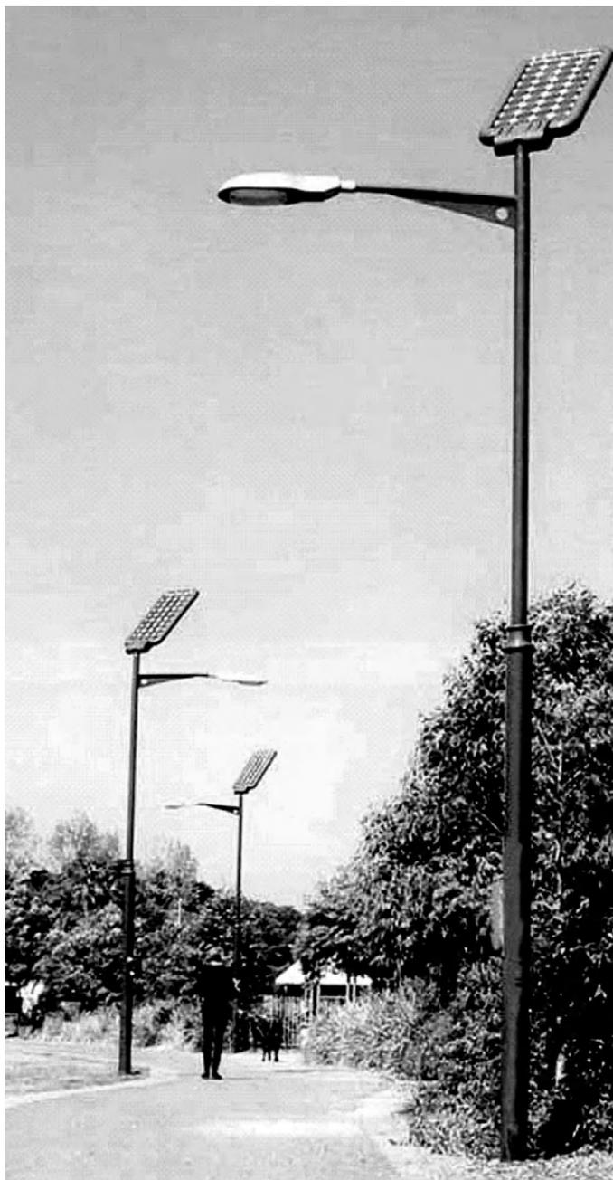
**FIGURE 9.26** Solar-powered LED street lighting with automatic on/off lasts for four to five nights after being fully charged. (Source: Hankey Asia.)
