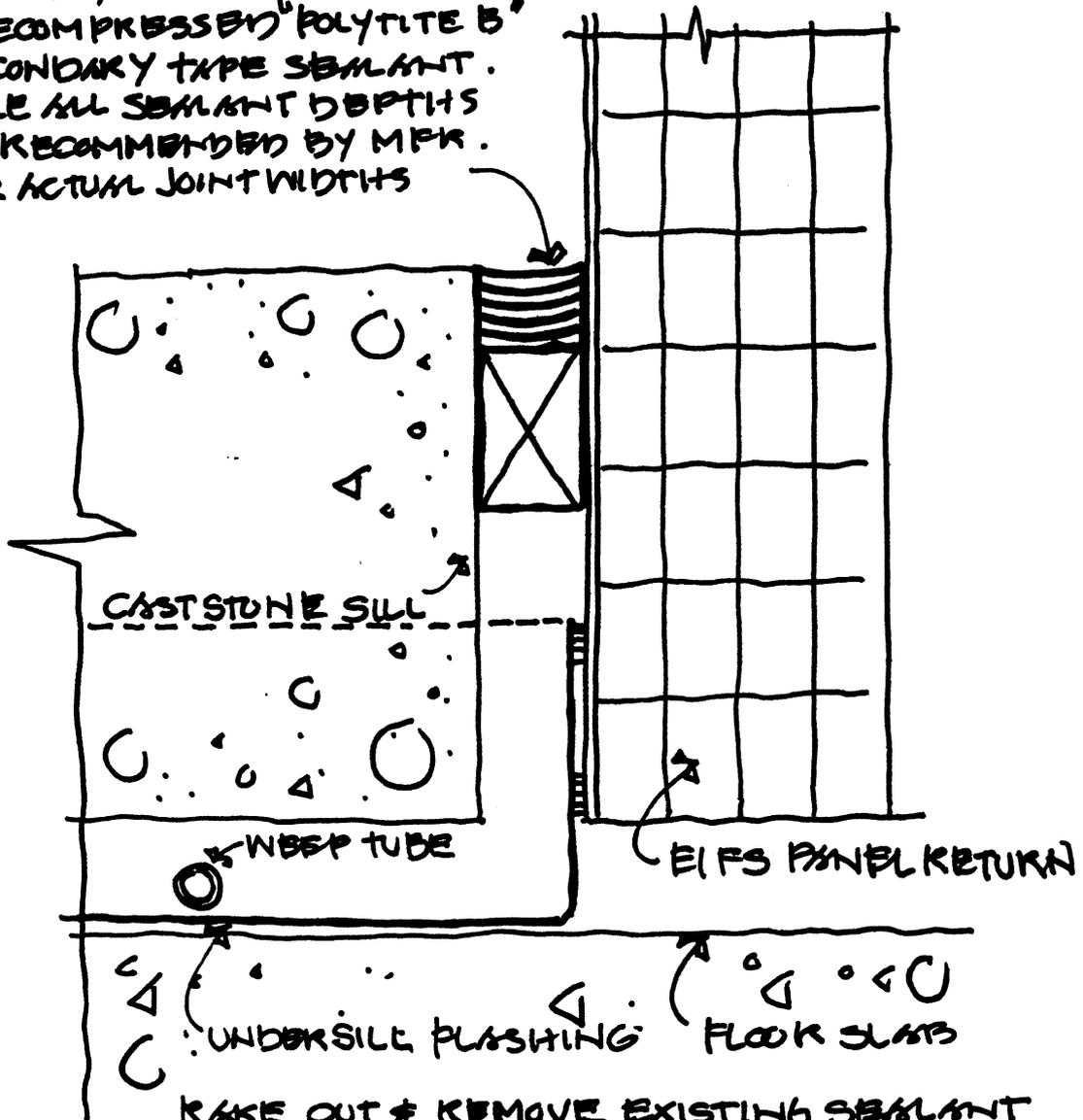
RAKE OUT & REMOVE EXISTING SEALANT
