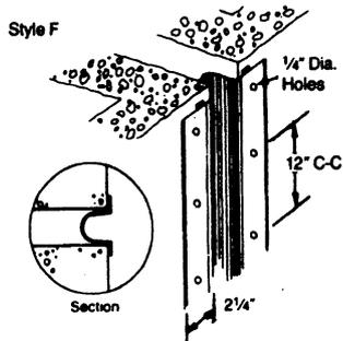
Sealant Transition for Abutment and Structural Joints
