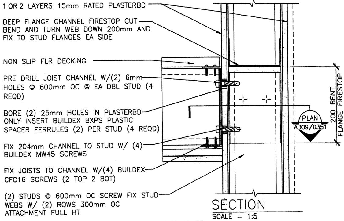
NOTE LIMIT TORQUE APPLIED TO PREVENT STRIPPING OF SCREWS & DETERMINE IF CONNECTION WILL PERFORM AS REQD
