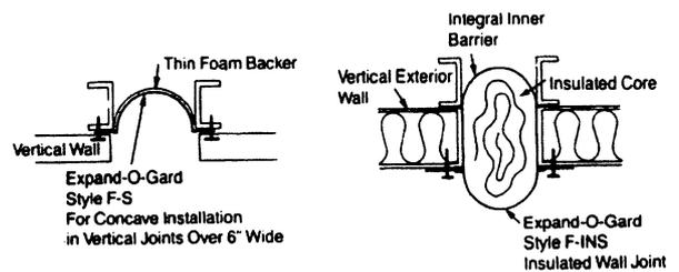
Fig. 12-23 Pictorial and detail views of various expansion joint systems [from manufacturer]
