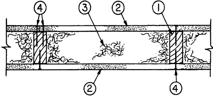
1. **Wood Studs** — Nominal 2 by 4 in. spaced 16 in. OC effectively fire-stopped.
