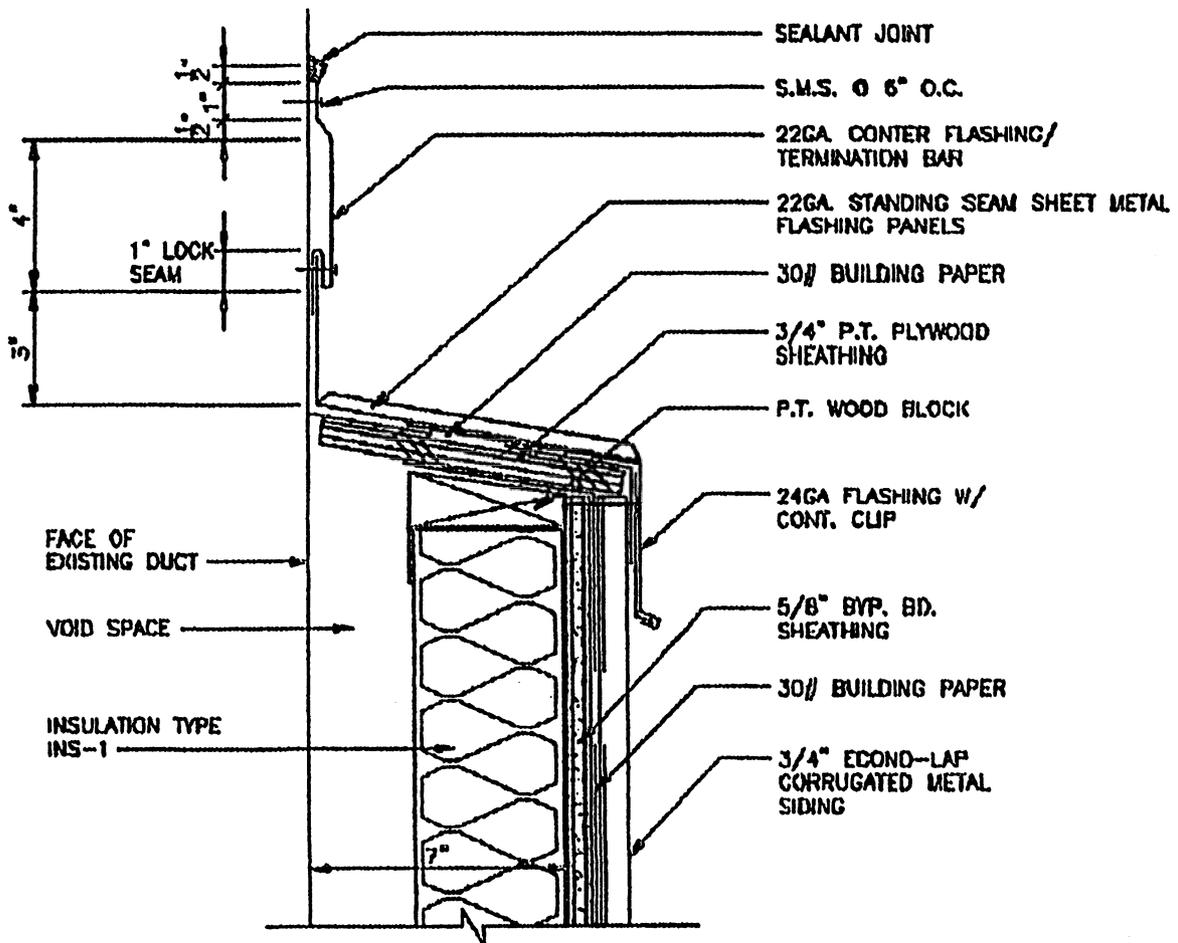
DUCT TO WALL FLASHING
