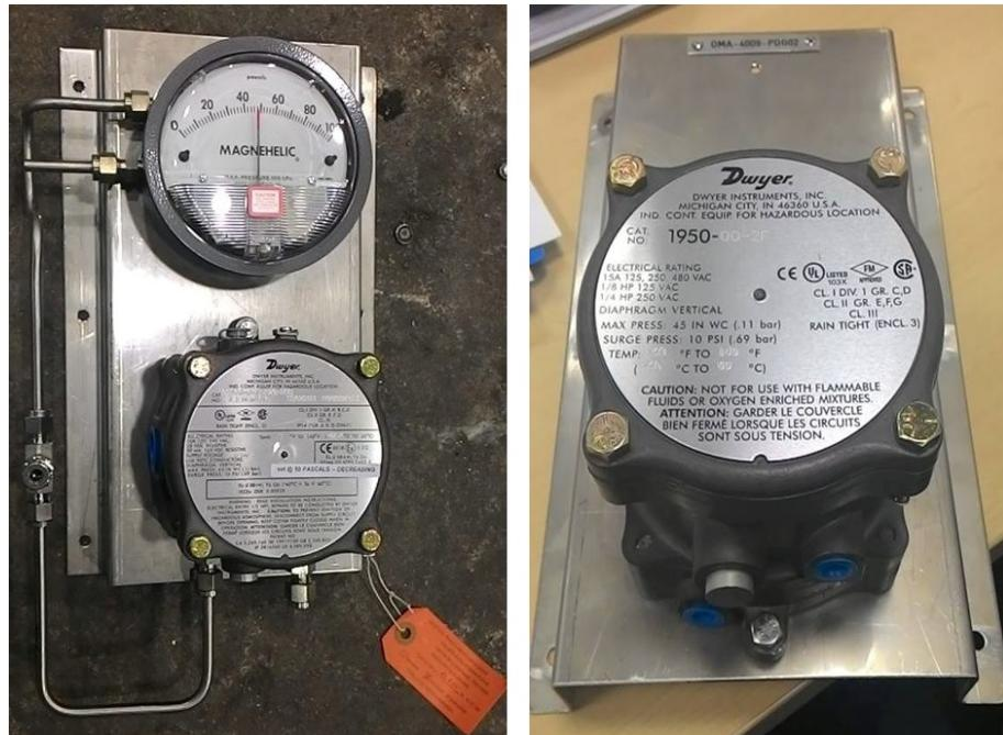
Fig.11.1. Differential pressure set & pressure switch alone
