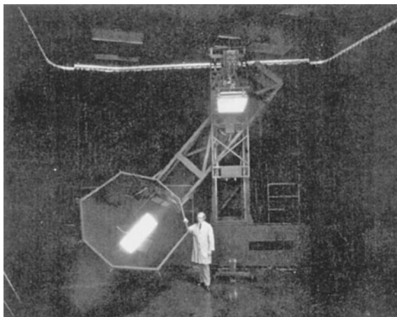
FIGURE 10.15 Mirror photometer used to measure the luminous intensity of a light source or luminaire in all directions. [General Electric Co.]
