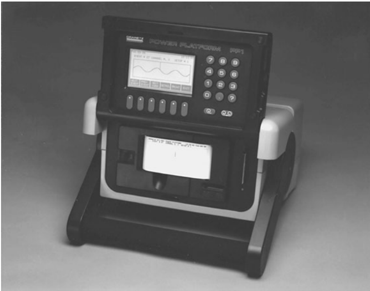
FIGURE 1.115 An eight-channel analyzer for capturing transients, voltage sags, swells, harmonics, and other power disturbances. Used in conjunction with the PQ Task Card®, the Power Platform® can generate reports and do K-factor computations for transformer selection. [Dranetz Technologies, Inc.]
