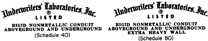
FIGURE 9.71 Identification of aboveground PVC conduits.
