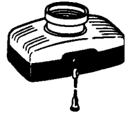
FIGURE 4.168 Porcelain-base lampholders for use with nonmetallic-sheathed cable.
