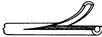
FIGURE 2.44 Another safe method of removing insulation from conductors is to peel the insulation back and then cut outward.
