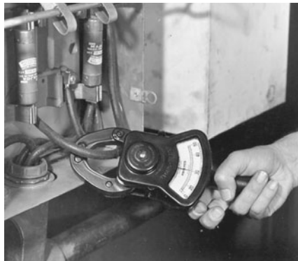
FIGURE 1.72 Application of a split-jaw ammeter. [Martindale Electric Co.]
