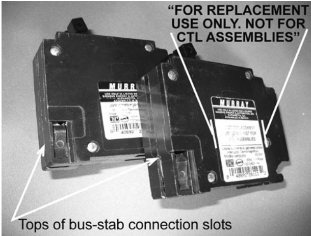
FIGURE 4.88 A 20-amp Class CTL tandem (left) and a non Class CTL tandem (right) circuit breaker shown for comparison. The CTL breaker set has a restricted-height bus connection slot (compare the dimension markings) that will only mount where a bus stab has been slotted by the panelboard manufacturer.
