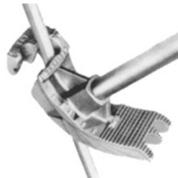
FIGURE 9.52D No. 9 Benfield double-grooved bender for \frac{1}{2} - \frac{3}{4} -in EMT and \frac{1}{2} -in rigid conduit. Note that the handle has a weatherproof Zip Guide plus an expanded end permitting its use as a stub straightener. [Jack Benfield, patent holder]
