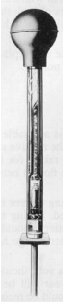
FIGURE 4.195 Hydrometer syringe. [Electric Storage Battery Co.]
