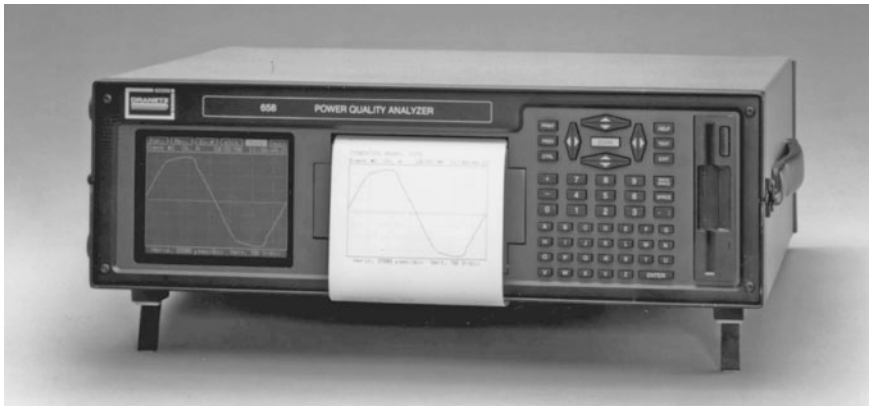
FIGURE 5.89 Analysis of power quality with a Model 658 digitizing oscilloscope, true RMS ammeter, true RMS voltmeter, harmonic distortion analyzer, power disturbance monitor, and strip chart recorder in one compact instrument. [Dranetz Technologies, Inc.]
