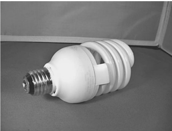
FIGURE 10.40 A new, twisted-tube CFL. As can be seen to the left, this one has a double-contact base, so it can operate at three different wattages.
