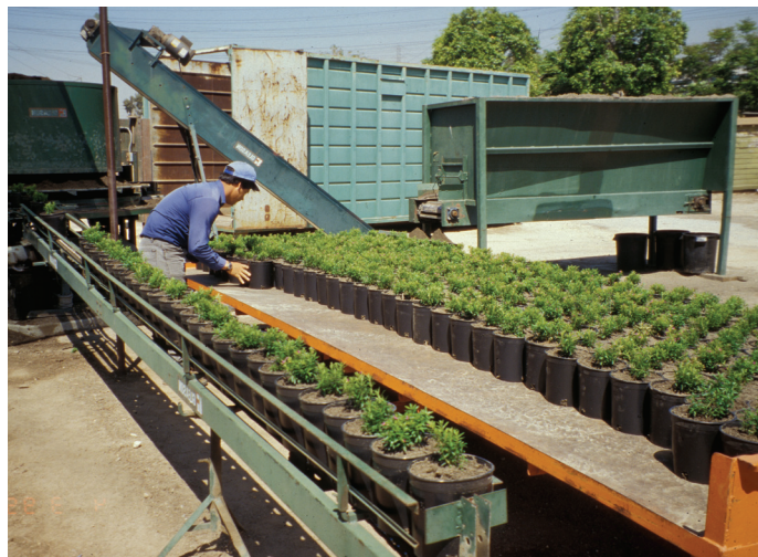
Automation in container nurseries can help workers in transplanting and movement of plant.
