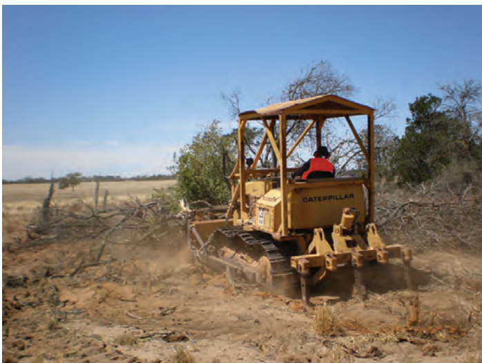
Figure 3. Tractor with three tines ripping a rabbit warren. Photo courtesy: S Edwards
