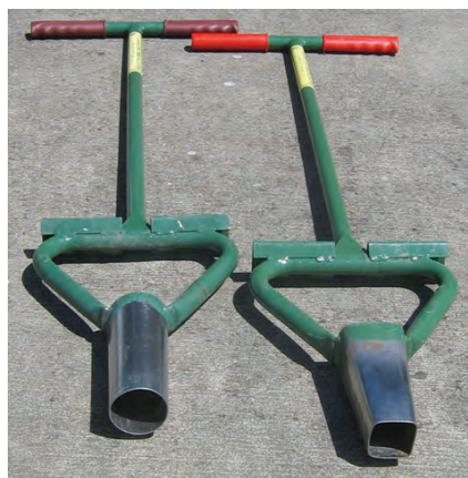
Figure 7. Hamilton tree planters with round or square ends for different shaped seedling tubes
