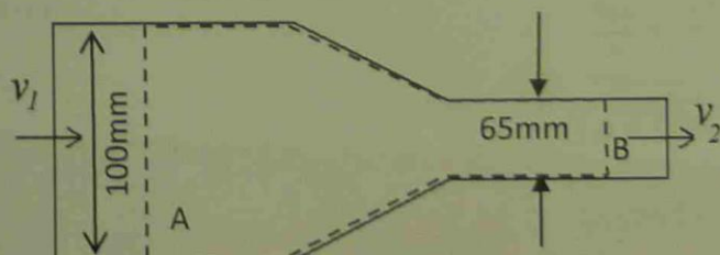
Figure Q4.1 control volume on a converging pipe section
