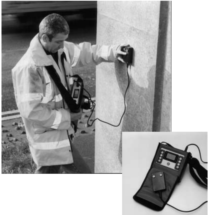
Figure 2.7 Reinforcement cover meter (courtesy of CMT Instruments).
