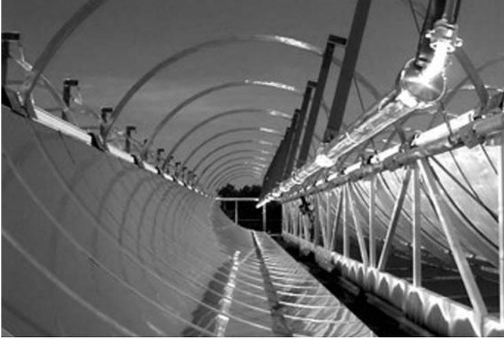
Figure 4.11 Parabolic reflector (Courtesy of Solargenix)
