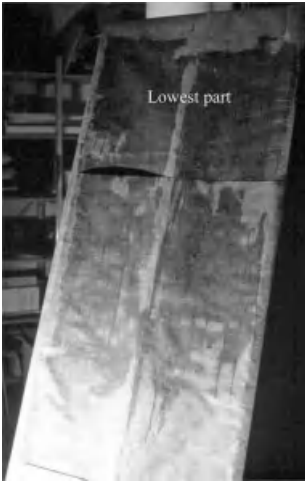
Figure 6.27. Cathedralized ceiling assembly 4, condensation on the underlay. Largest deposit at the lowest part of the underlay.
