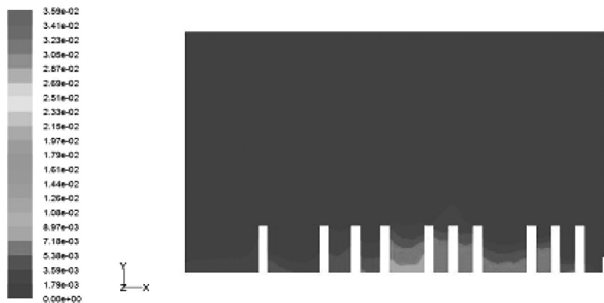
FIGURE 5.23 Contours of CO mole fraction \text{kmol/m}^3 at z = 12.15 m.
