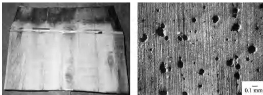
Figure 7.14. Corroded underside of a zinc/titanium cover.
