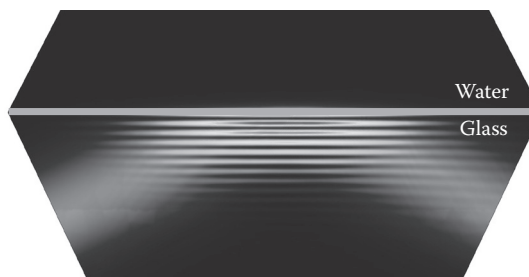
FIGURE 3.4 COMSOL simulation of total internal reflection in Figure 3.3. Plotted in the figure is time-averaged total electromagnetic energy density in the vicinity of the glass–water interface. Because the refractive indices of glass and water are 1.515 and 1.33, respectively, total internal reflection occurs at \theta > \theta_{cr} = 61.39^\circ . In this figure, the incident angle of the incoming Gaussian illumination beam is \theta = 64.54^\circ , and the illumination wavelength is 514 nm.
